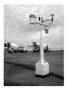
Figure 8.2 Weather station (records temperature, humidity, and wind speed)
