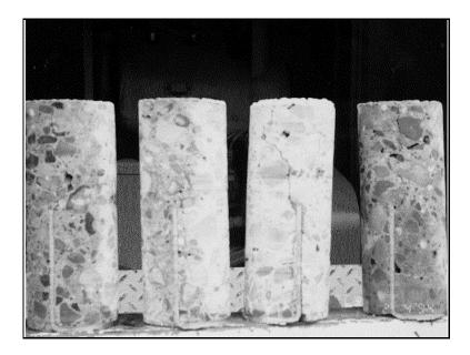
Figure 3.2 Cores from nonsawcut part in subsection 1 where Type I crack inducer was located
