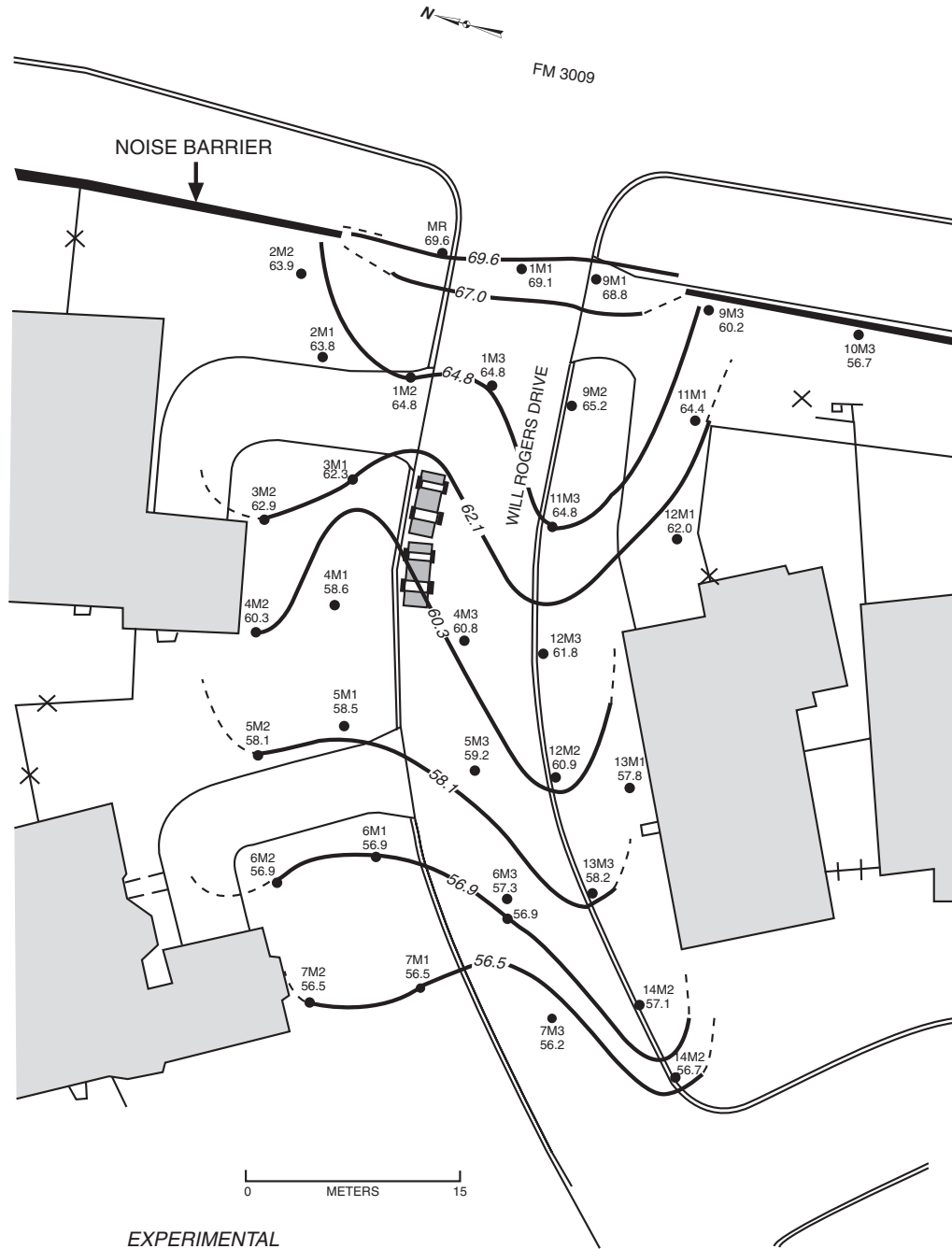
Figure 4.7 Constant noise level contours — Field measurements on Will Rogers Drive at FM 3009
