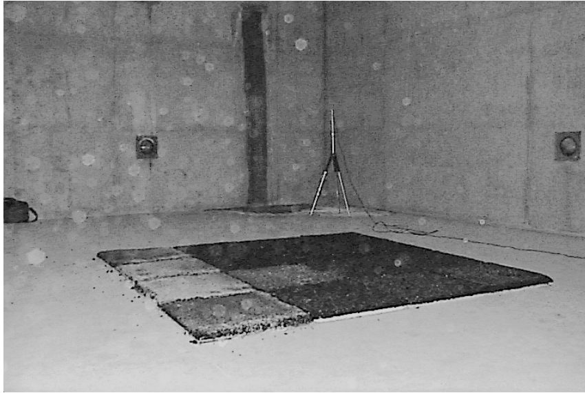
Figure 4.2. Photo showing test sample in reverberation room, with microphone in the background.
