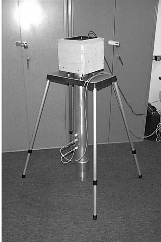
Figure 5.4. Impedance tube with stand for measuring acoustical absorption of flat surfaces.
