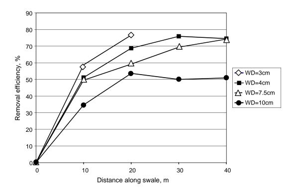
Figure 3.7 Effect of Water Depth and Swale Length on TSS Removal Efficiency
