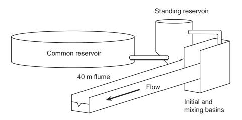
**Figure 3.3 General Flume Apparatus**
