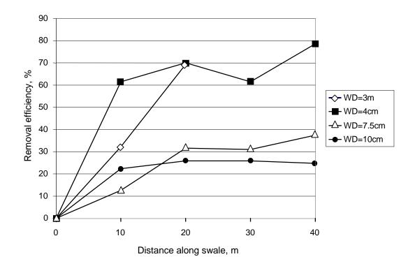
Figure 3.8 Effect of Water Depth and Swale Length on COD Removal Efficiency
