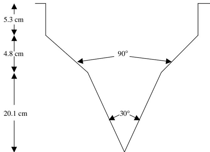
**Figure 4.3 Compound V-Notch Weir for Flow Measurement**
