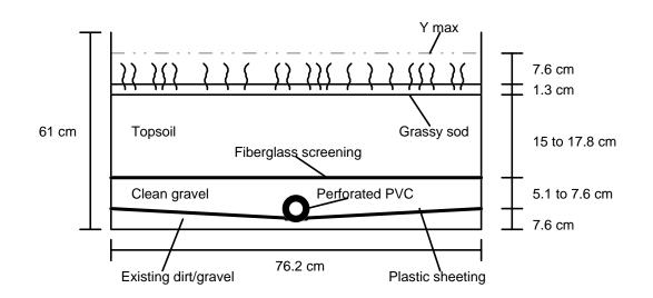
Figure 3.1 Cross Section of Channel Swale
