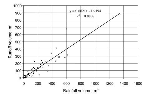
Figure 4.5 Initial Calculation of Runoff Coefficient of Filter Strip Drainage Area, US 183
