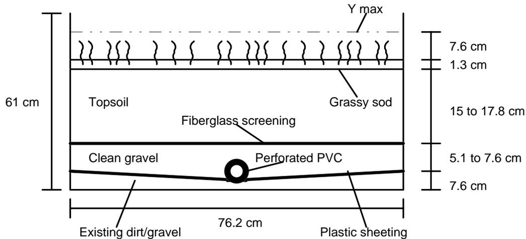
**Figure 3.1 Cross Section of Channel Swale**
