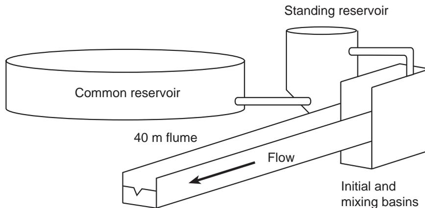
**Figure 3.3 General Flume Apparatus**
