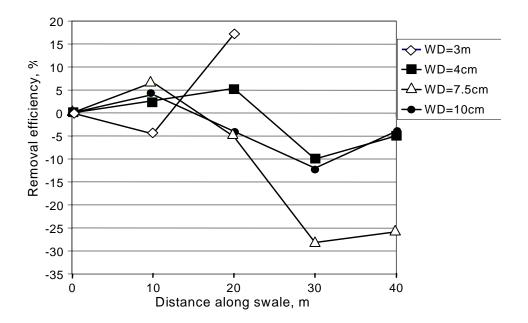
Figure 3.9 Effect of Water Depth and Swale Length on Nitrate Removal Efficiency
