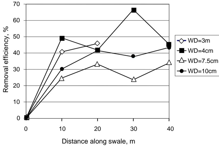
**Figure 3.11 Effect of Water Depth and Swale Length on TP Removal**
