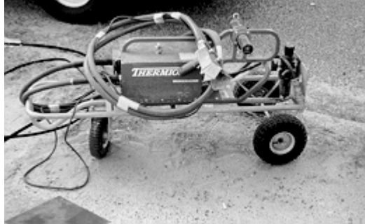
Figure 5.5: Arc spraying equipment
