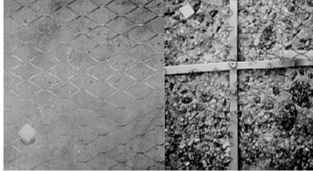
Figure 5.14: Concrete surface preparation comparison. Figure on left represents the lightly sandblasted surface used in the first two trials. The right figure shows exposed aggregates from heavier sandblasting used in the third trial.
