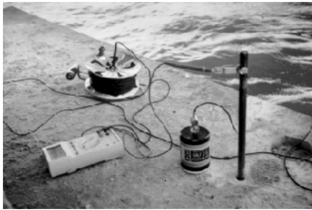
Figure 4.7: Setup for half-cell potential measurements
