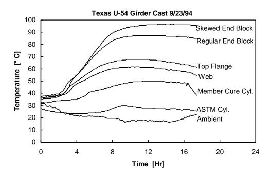
Figure 4.3 HPC temperature profile with 4-hour pre-set
