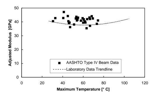
Figure 5.13 Comparison of modulus of elasticity data from the laboratory and field
