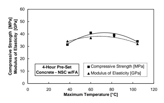
Figure 4.9 Release data for NSC with fly ash cured with a 4-hour pre-set period
