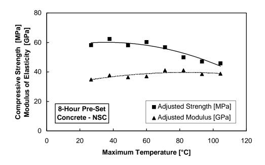
Figure 4.13 Twenty-eight-day data for NSC match/air cured cylinders
