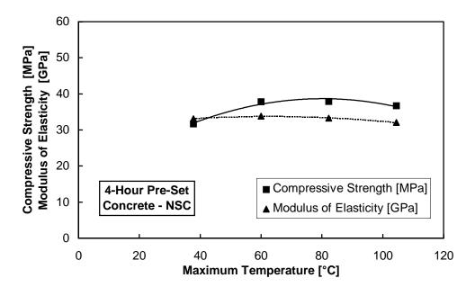
Figure 4.7 Release data for NSC cured with a 4-hour pre-set period
