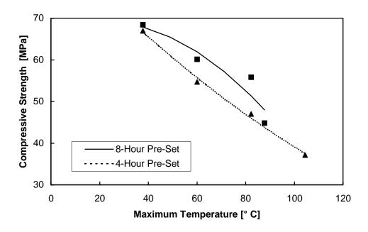
Figure 5.8 Compressive strength decrease of 8-hour and 4-hour pre-set specimens for the NSC mix with fly ash
