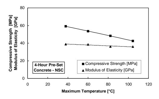
Figure 4.15 Twenty-eight-day data for NSC match/moist cured cylinders with a 4-hour preset period
