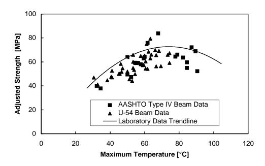
Figure 5.5 Comparison of compressive strength data for laboratory and field specimens
