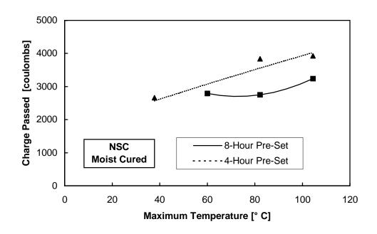
Figure 5.16 Permeability data for moist cured NSC without fly ash
