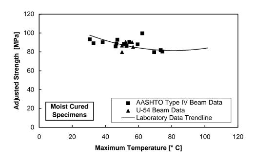
Figure 5.11 Comparison of moist cured design strength data from the laboratory and field
