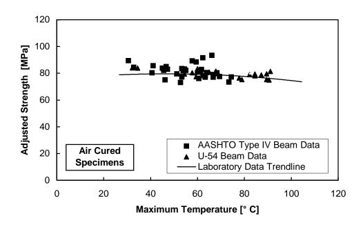
Figure 5.10 Comparison of air cured design strength data from the laboratory and field
