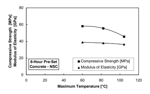
Figure 4.14 Twenty-eight-day data for NSC match/moist cured cylinders
