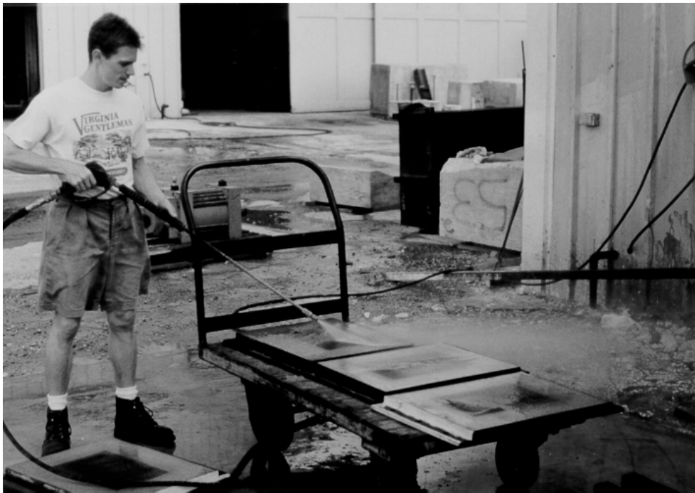
Figure 4- 2 Cleaning of concrete platens
