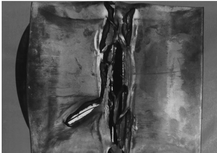
Figure 7-6 Fractured reinforcing steel shims
