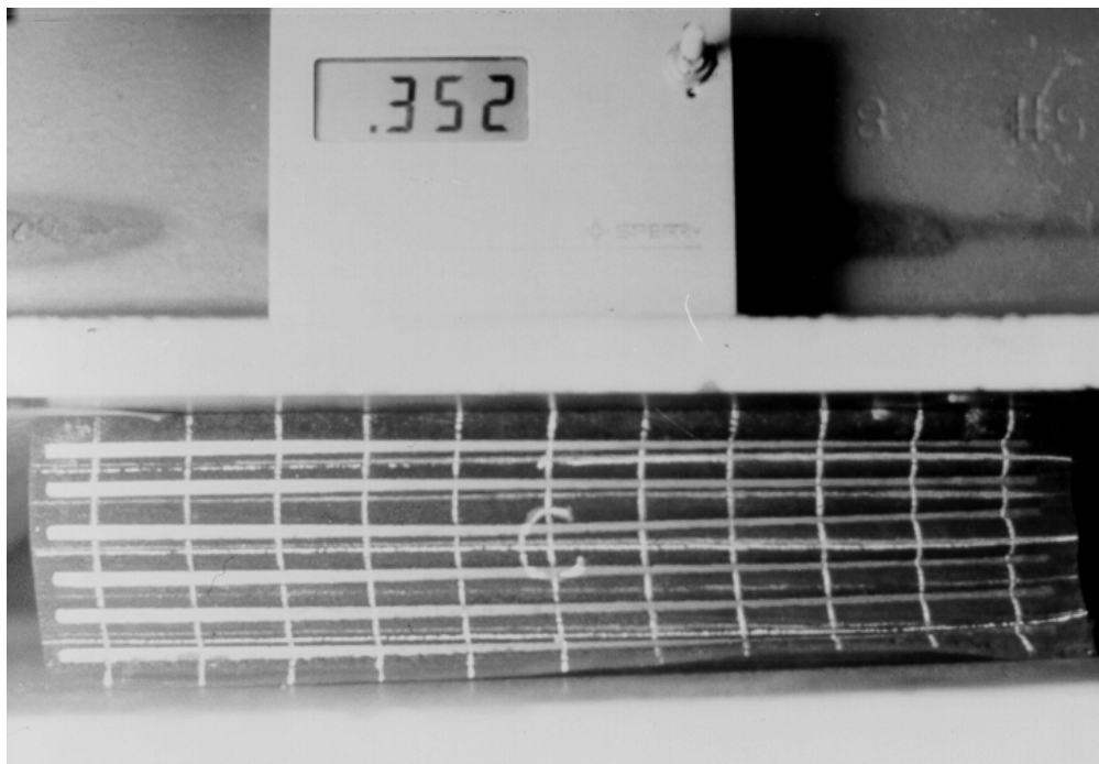
Figure 4- 23 Bearing exhibiting lift-off at 7.69 MPa (1100 psi)
