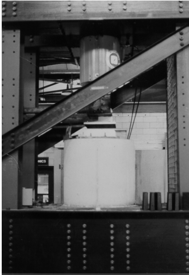
Figure 7- 1 Compression failure test apparatus
