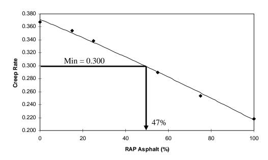
Figure 4.4 Creep rate trend for RTFO and PAV-aged DG blend at -12°C
