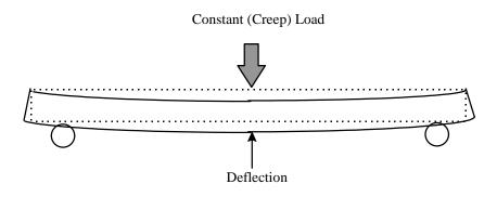
Figure 2.6 Bending beam rheometer loading geometry
