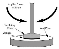
Figure 2.4 Dynamic shear rheometer loading geometry
