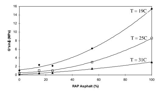
Figure 3.6 G\*sin trend for RTFOT and PAV-aged AF blend
