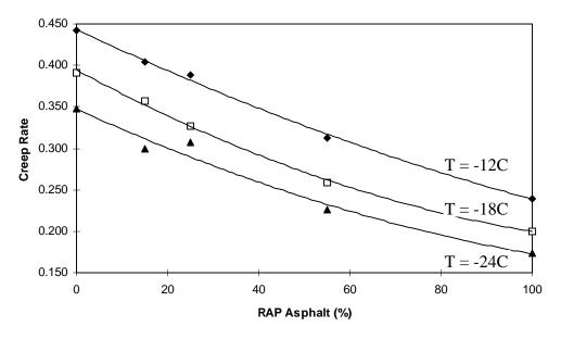
Figure 3.10 Creep rate trend for RTFOT and PAV-aged AF blend
