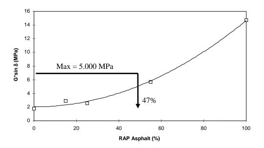
Figure 4.5 G\*sin trend for RTFO and PAV-aged DG blend at 25°C
