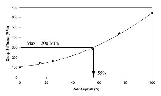
Figure 4.3 Creep stiffness trend for RTFO and PAV-aged DG blend at -12°C
