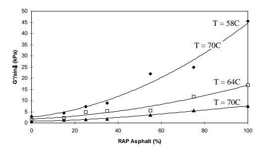
Figure 3.2 G\*/sin trend for unaged MF blend
