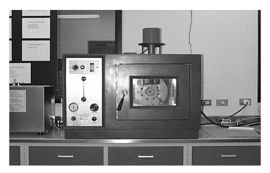
Figure 2.1 Rolling thin film oven
