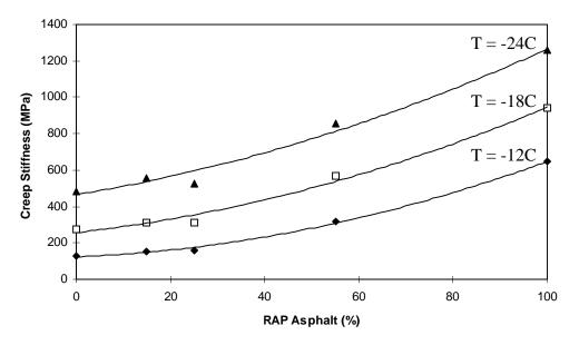
Figure 3.7 Creep stiffness trend for RTFOT and PAV-aged CG blend
