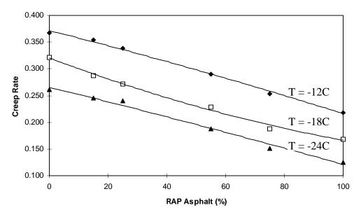
Figure 3.9 Creep rate trend for RTFOT and PAV-aged DG blend
