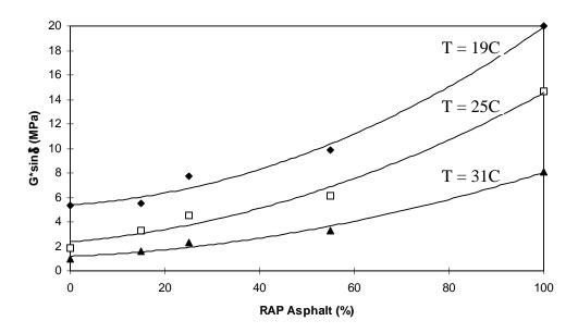
Figure 3.5 G\*sin trend for RTFOT and PAV-aged MG blend
