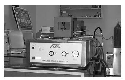
Figure 2.5 Bending beam rheometer
