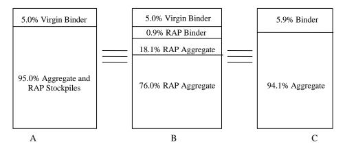
Figure 4.7 Schematic view of material components in the mix
