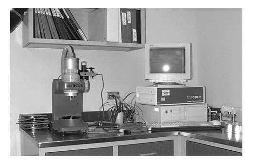
Figure 2.3 Dynamic shear rheometer
