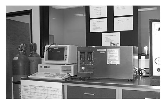
Figure 2.2 Pressure Aging vessel
