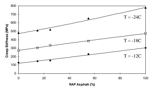
Figure 3.8 Creep stiffness trend for RTFOT and PAV-aged CF blend
