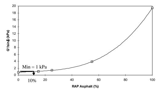
Figure 4.1 G\*/sin $\delta$  trend for unaged DG blend at 64°C
