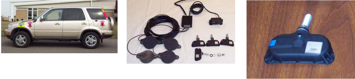
Figure 3.12 – System I Test Vehicle / System I Display and Tire Sensor-Transmitter
