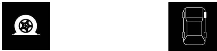
Figure 10.1 – Suggested icon for indication of significant tire underinflation and alternative vehicle-based display.
