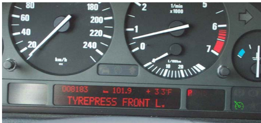
Figure 7.6 – Visual Warning of System E
