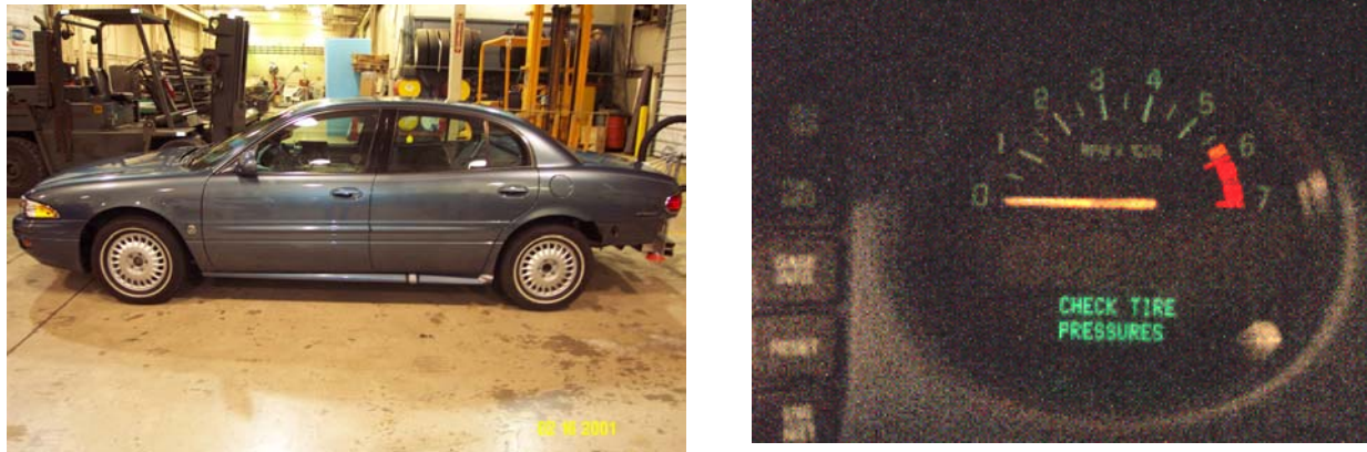
Figure 3.2 – System B Test Vehicle / TPMS Warning Message
