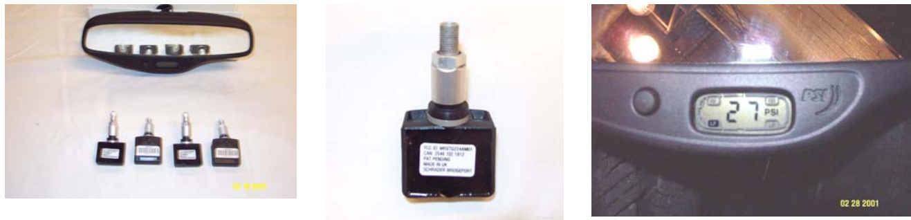
Figure 3.11 – System H Sensor-Transmitter / Rearview Mirror Display
