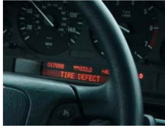
Figure 3.3 – System C Test Vehicle / TPMS Warning Message
