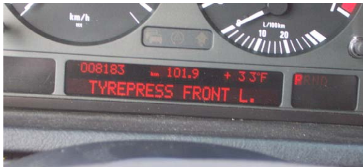
Figure 3.7 – System E TPMS Warning Message With Wheel Location
