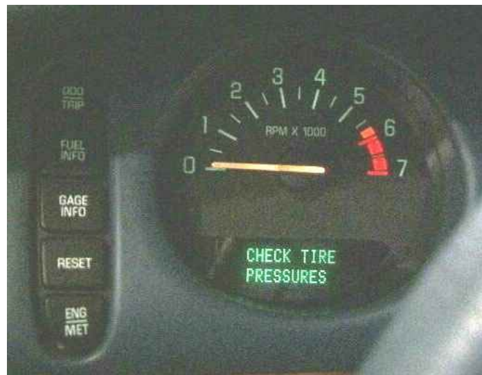
Figure 7.2 – Visual Warning of System B
