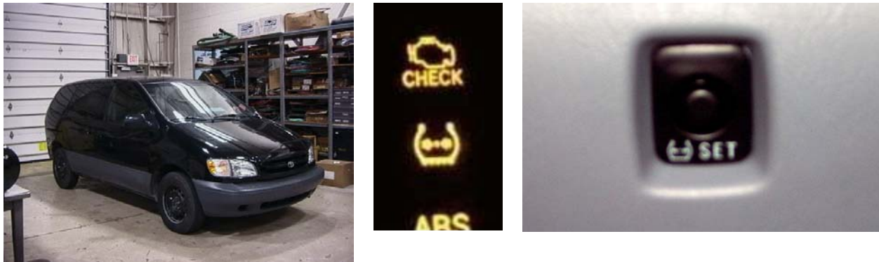
Figure 3.5 – System D Test Vehicle / Warning Light (Middle) / TPMS Reset Button
