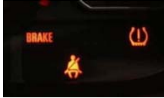
Figure 3.1 – System A Test Vehicle / Significant Underinflation Warning Light (Rightmost)
