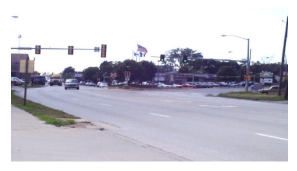
Figure 2: State Street (US Highway 67) after the addition of a continuous two-way left-turn lane
