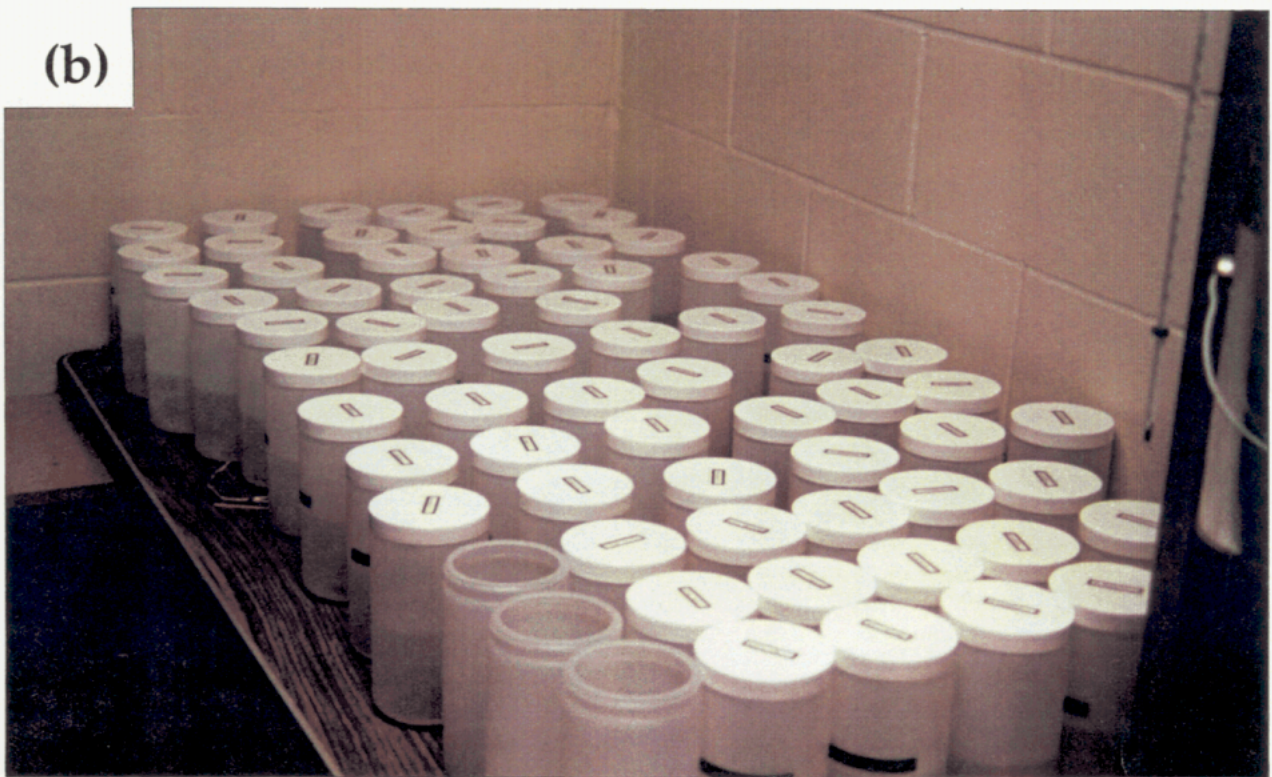
Figure 1. A cone-shaped concrete sample (a) in the test cell (b) for concrete degradation by corrosion-inhibitor-added deicing salts.
