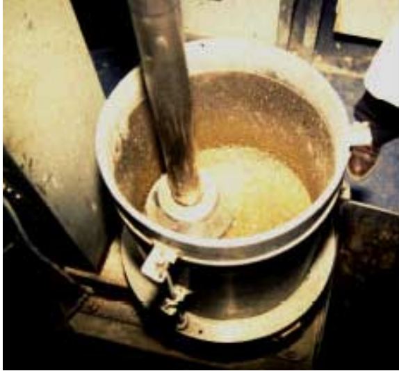
Figure 7. QMOT test equipment for moisture density test.
