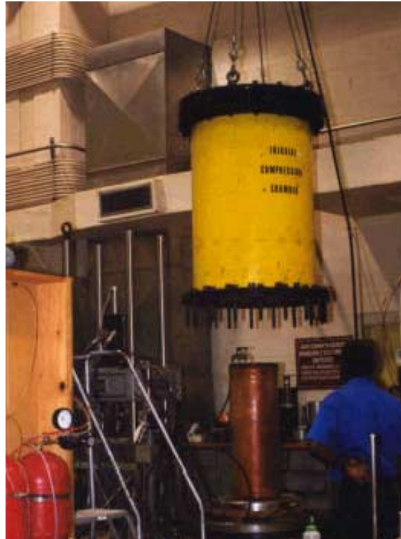
Figure 11. Placement of triaxial chamber around test specimen.
