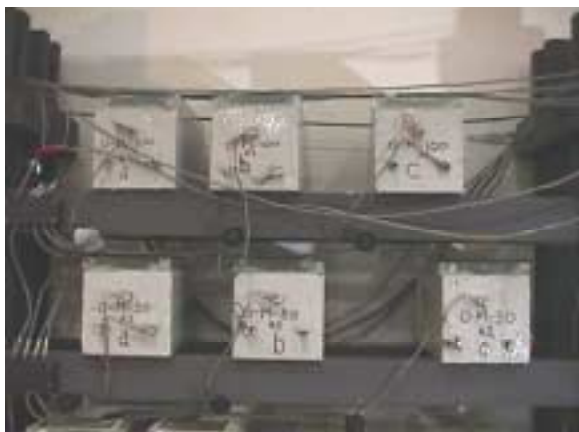
Figure A9. Photograph of pre-cracked concrete minibeam tests.
