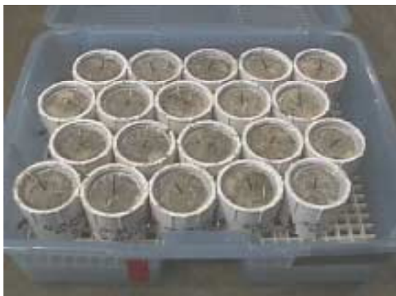
Figure A5. Photograph of fixed chloride test specimens in humidity container.
