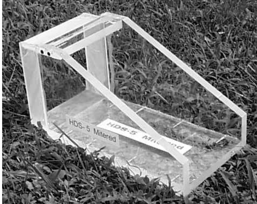
Figure 6. Culvert model 1, HDS-5 chart 8, scale 3.
