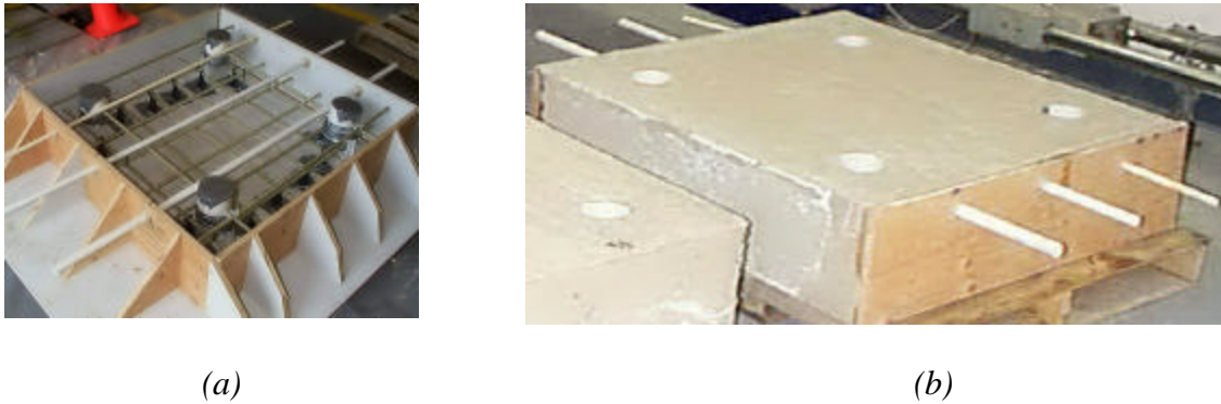
Figure 6. Variable-diameter PVC pipe specimen: (a) before casting and (b) after casting.
