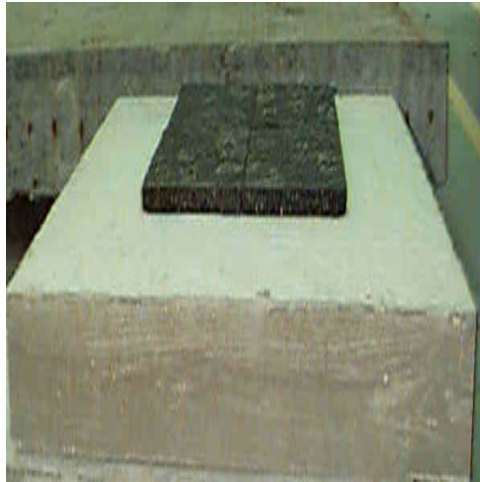
Figure 12. Simulated asphalt overlay configuration.
