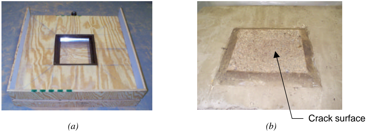
Figure 3. (a) A custom made concrete form with a steel concrete cracking mechanism and (b) one of the two crack surfaces created after the specimen had been cracked into two pieces.
