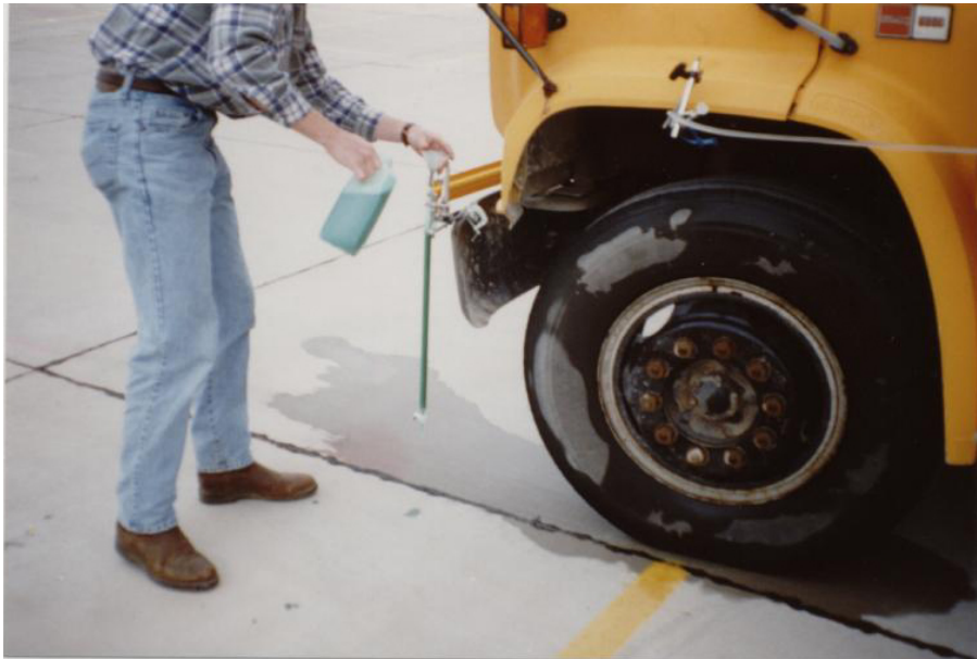
FIGURE 2 Burettes on Bus Body and Tire Water Spraying Apparatus
