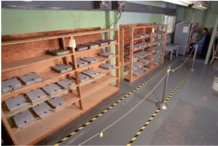
Figure 5.2: Laboratory electrochemical aging of the five thermal-sprayed titanium anodes on concrete slabs.
