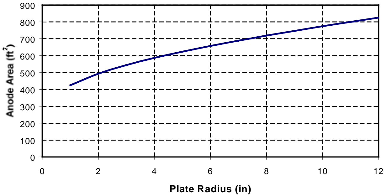
Figure B.2: Allowable titanium surface area vs. plate size - inches.
