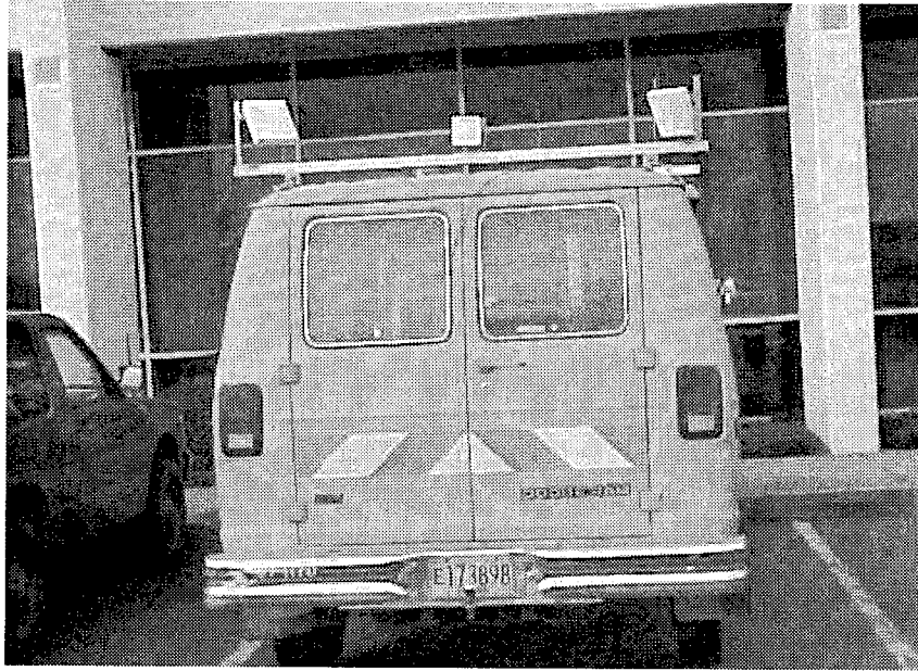
Figure 2.2: The patch antennas, mounted on the rear light bar of the van.
