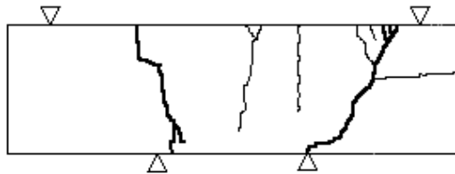
Figure B.10.2.3: Typical failure modes for Owens Corning/Reichhold beams reinforced for flexure plus shear at 90 degrees.
