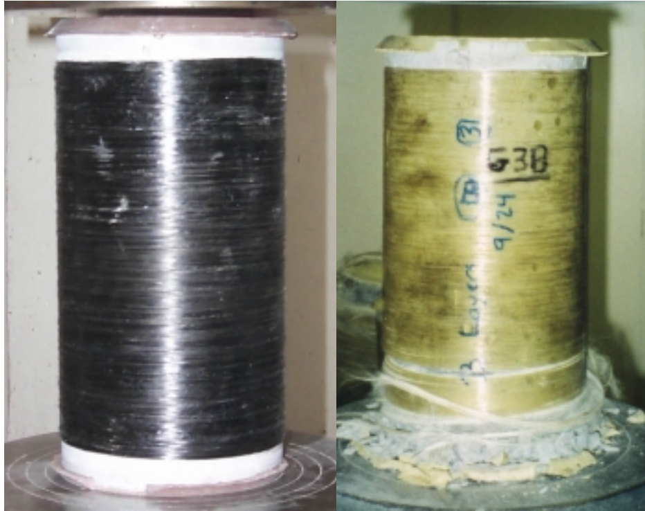
Figure 3.16: Typical appearance of CFRP (left) and GFRP reinforced cylinder, broken (right).
