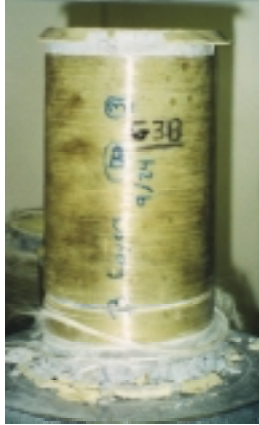
Figure 4.53: Typical Owens Corning/Reichhold reinforced cylinder after failure.
