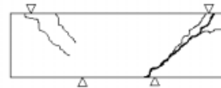
Figure B.2.1.3: Typical failure modes and crack patterns for flexurally reinforced MBrace™ carbon beams.
