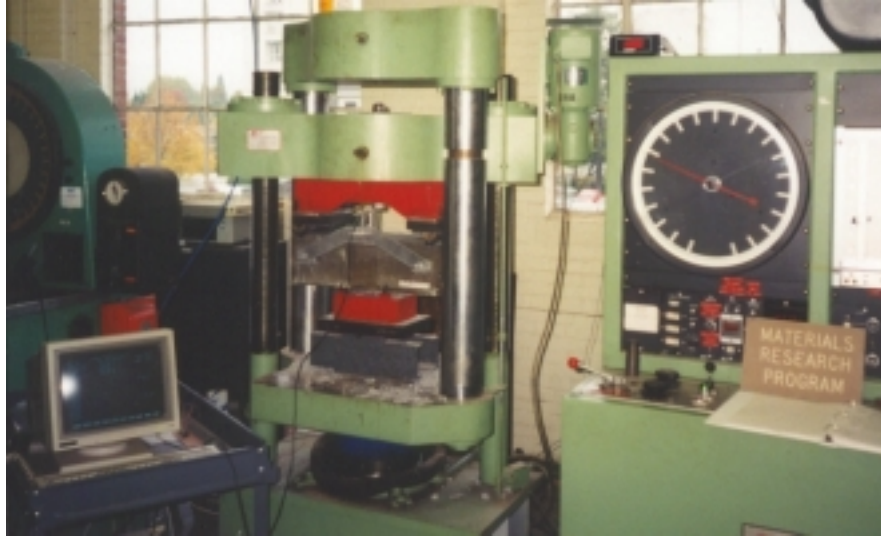
Figure 2.5: Beam test setup (Satec 200HVL universal testing machine).
