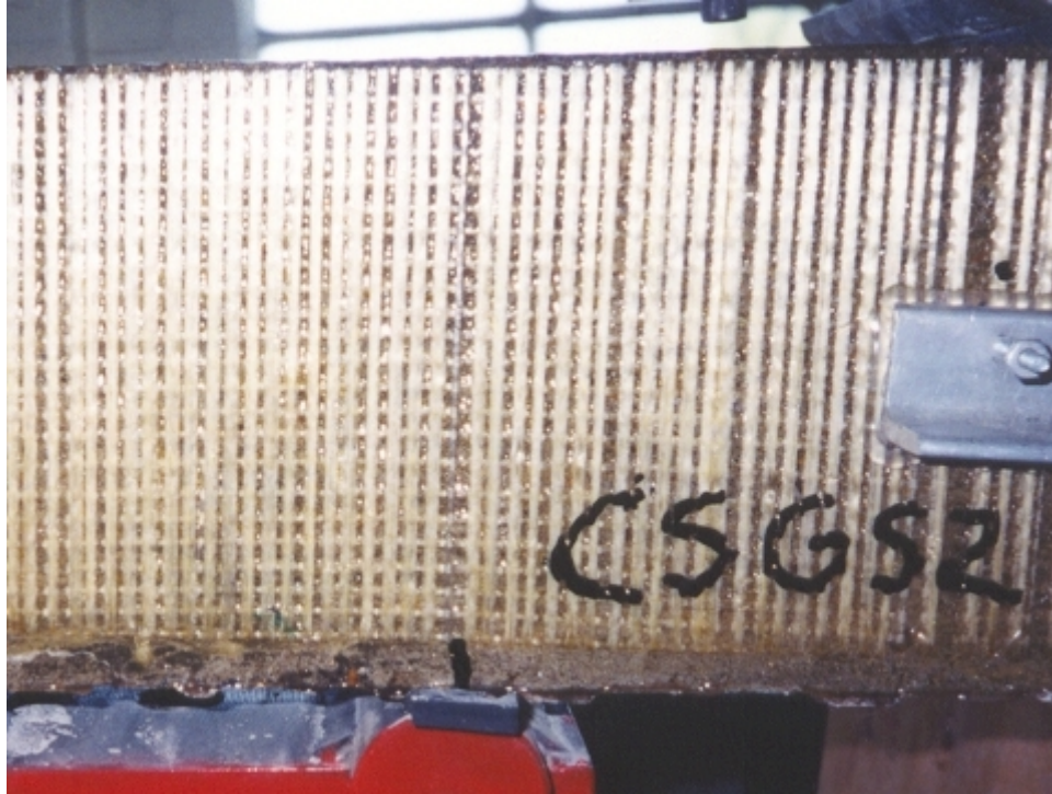
Figure 3.14: Typical appearance of Clark Schwebel Structural Grid.
