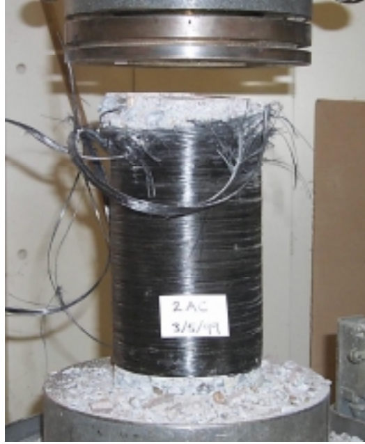
Figure 4.54: Typical Fortafil/Reichhold reinforced cylinder after failure.
