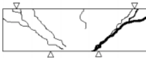
Figure B.5.1.3: Typical cracking and failure modes for beams reinforced for flexure with Tyfo® carbon FRP.
