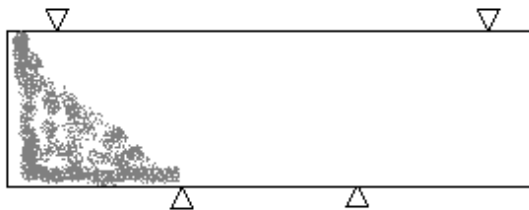
Figure B.8.3.4: Typical failure mode of beams strengthened with the Tyfo® glass system for shear at 45°.
