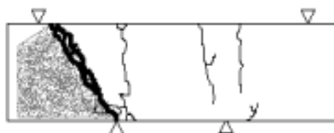
Figure B.10.3.3: Typical failure modes for Owens Corning/Reichhold beams reinforced for flexure and shear at 45 degrees.
