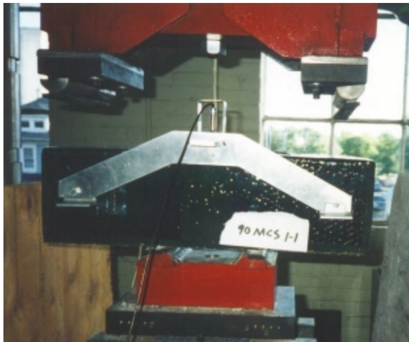
Figure 2.6: Third point loading frame.
