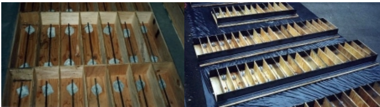
Figure 2.1: Molds used for preparation of reinforced concrete beam specimens.
