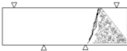
Figure B.6.4.2: Typical failure modes for CMI/Reichhold beams reinforced for shear at 45 degrees.
