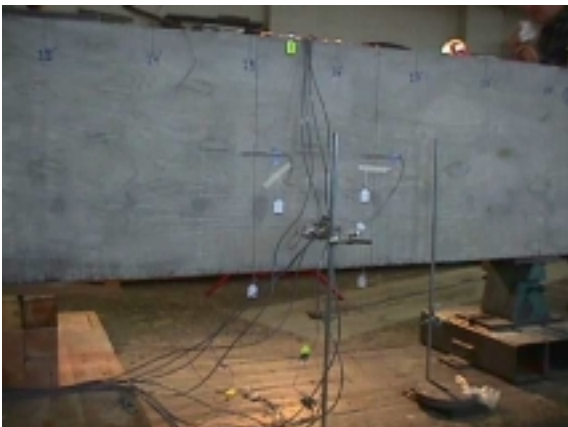
Figure A-21: Control beam shear sections
