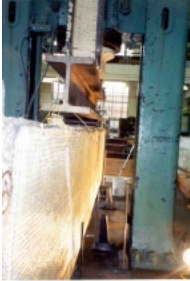
Figure A-45: Visible S&F beam deflections
