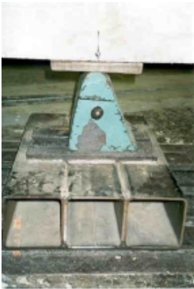
Figure A-26: Support point: rotation at failure
