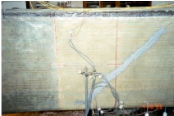
Figure A-46: S&F beam shear sections
