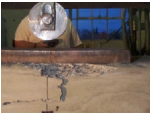
Figure A-27: Load point: crushing at failure
