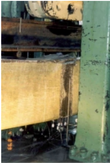
Figure A-41: Failure of Shear-only
