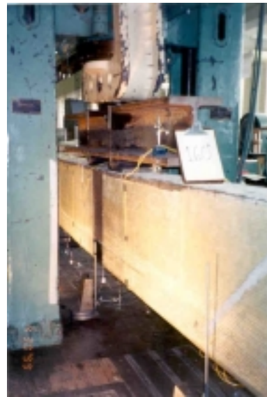
Figure A-48: Increase moment max. loading
