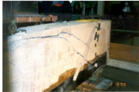
Figure A-29: Failure of Flexure-only beam
