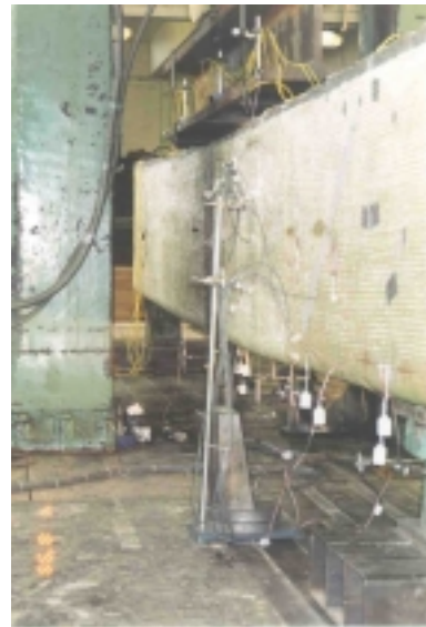
Figure A-44: S&F deflection under high load
