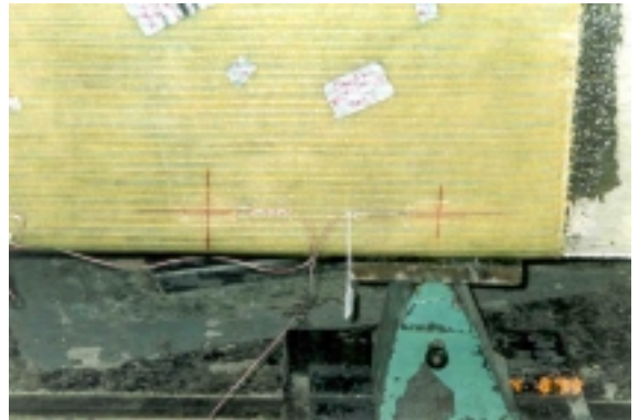
Figure A-43: Shear-only beam support point
