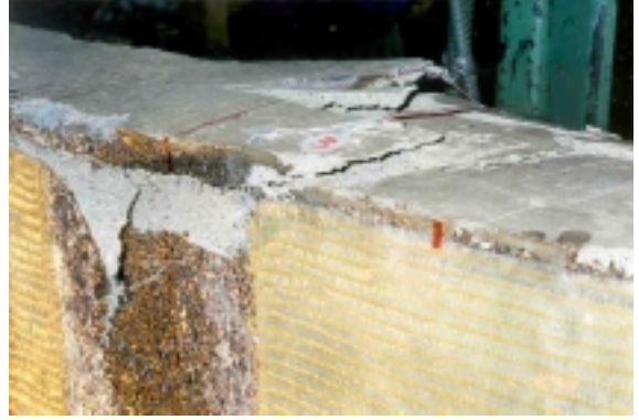
Figure A-42: Concrete crushing at midspan
