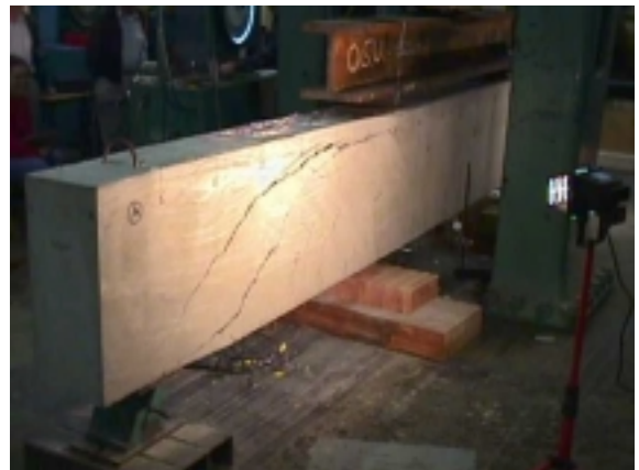
Figure A-24: Completed shear failure
