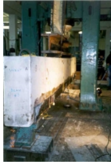
Figure A-28: Flexure-only beam testing
