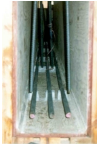
Figure A-6: Replicated steel reinforcing
