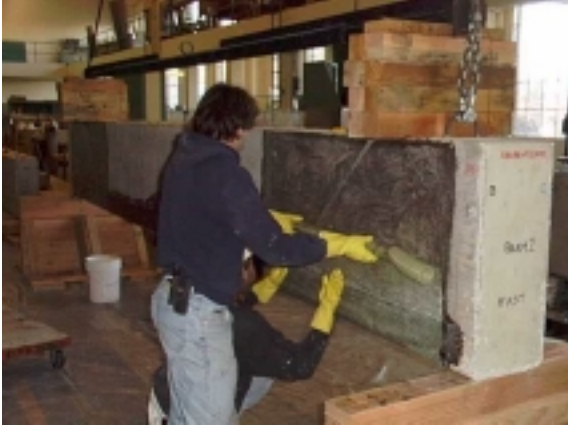
Figure A-13: GFRP application to test beams
