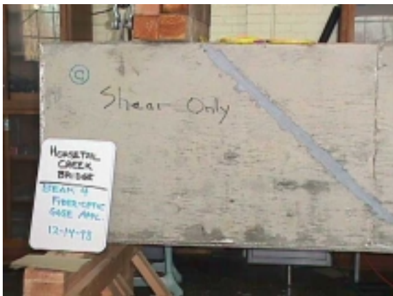
Figure A-9: Fiber optic gauge placement
