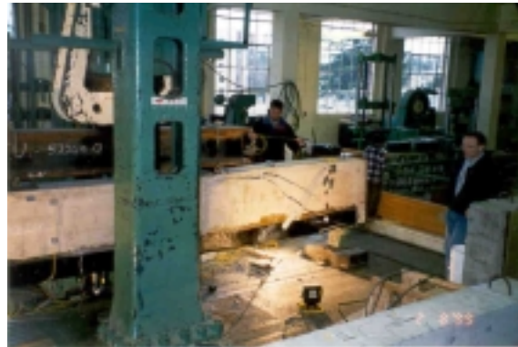
Figure A-35: Flexure-only beam at failure
