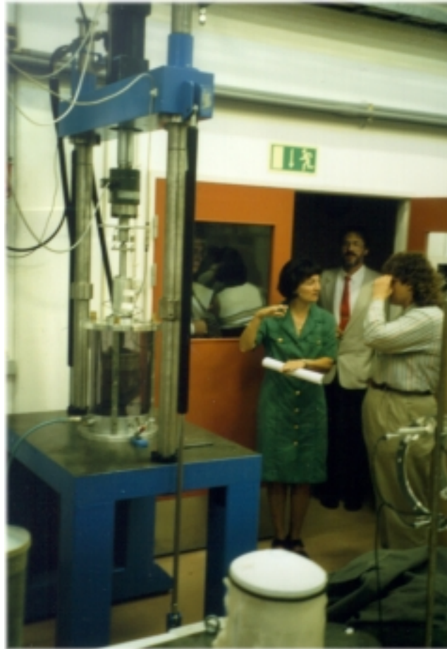
Figure 6. Triaxial testing machine at VTI.
