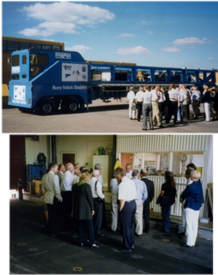
Figure 5. The (a) Heavy Vehicle Simulator and (b) a fully instrumented pavement test section in the pavement bay at VTI.
