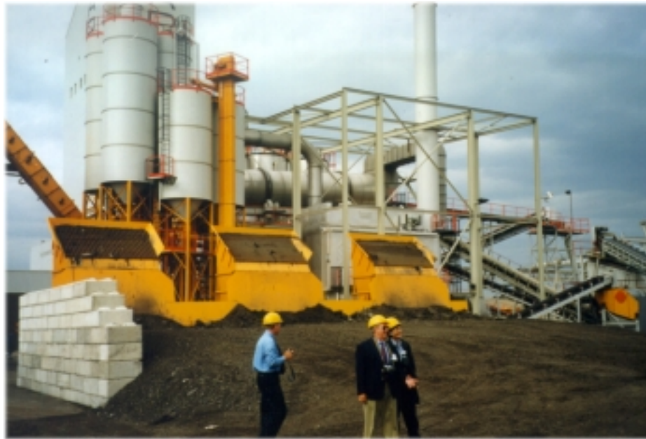
Figure 23. RAP is sorted before introduction into the lower drum at the Swiss-designed Ammann double drum asphalt plant in the Netherlands.
