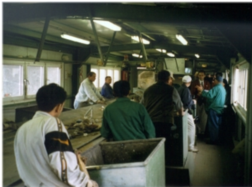
Figure 16. The sorting conveyor at the Remex C&D processing plant. Hand sorting is used to recover glass, metal, wood, cardboard, and plastic that is co-mingled with the C&D waste.
