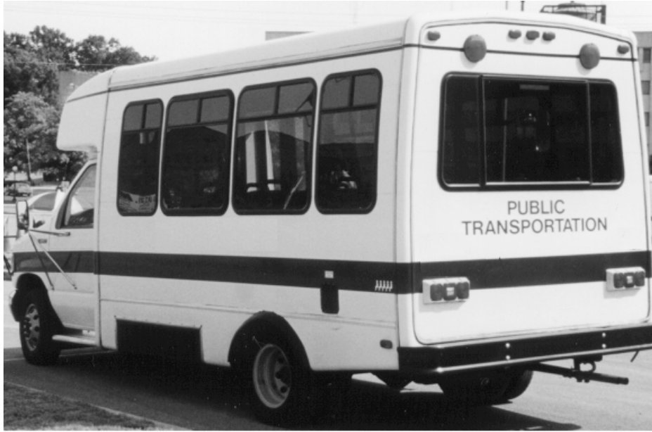
Figure 1 Cut-away chassis rural transit vehicle
