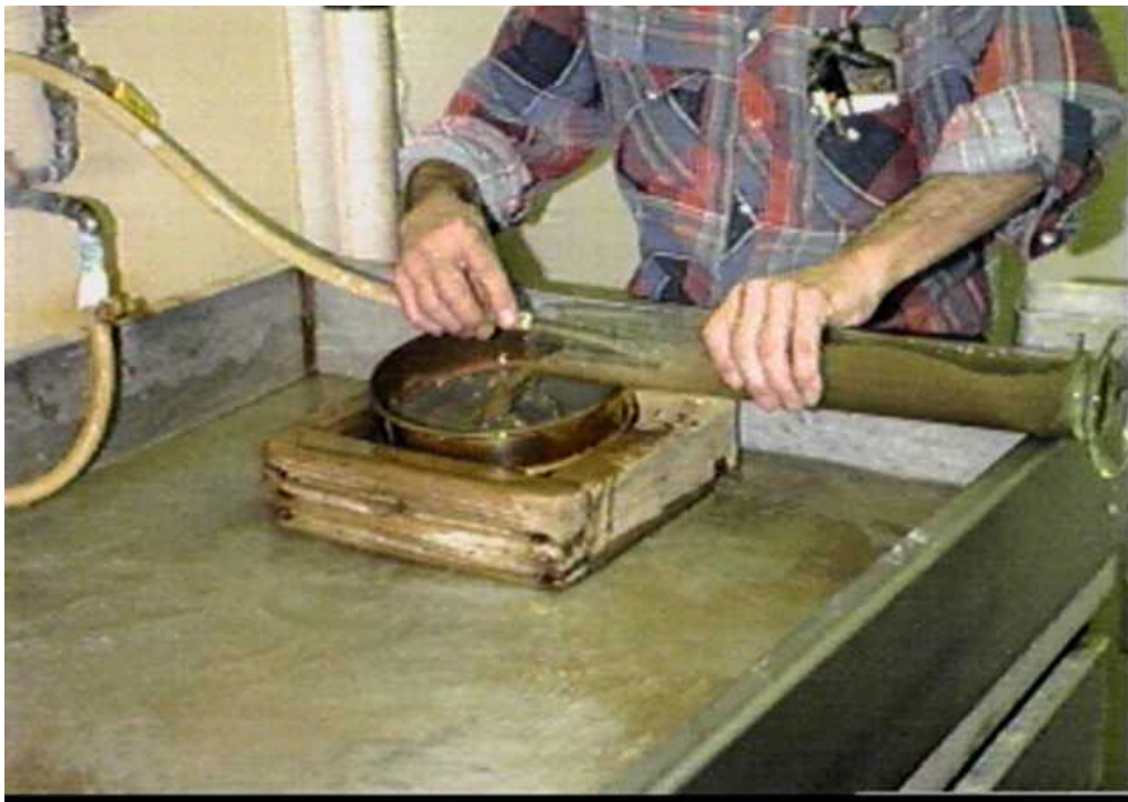
Figure 5: Pouring finished hydrometer from sedimentation over 0.075 mm sieve.
