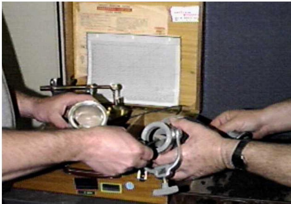
Figure 2. Placing calcium carbide into moisture tester chamber.
