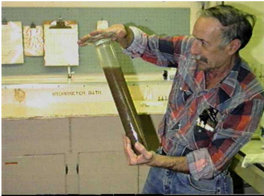
Figure 3: Agitating slurry in the sedimentation cylinder.
