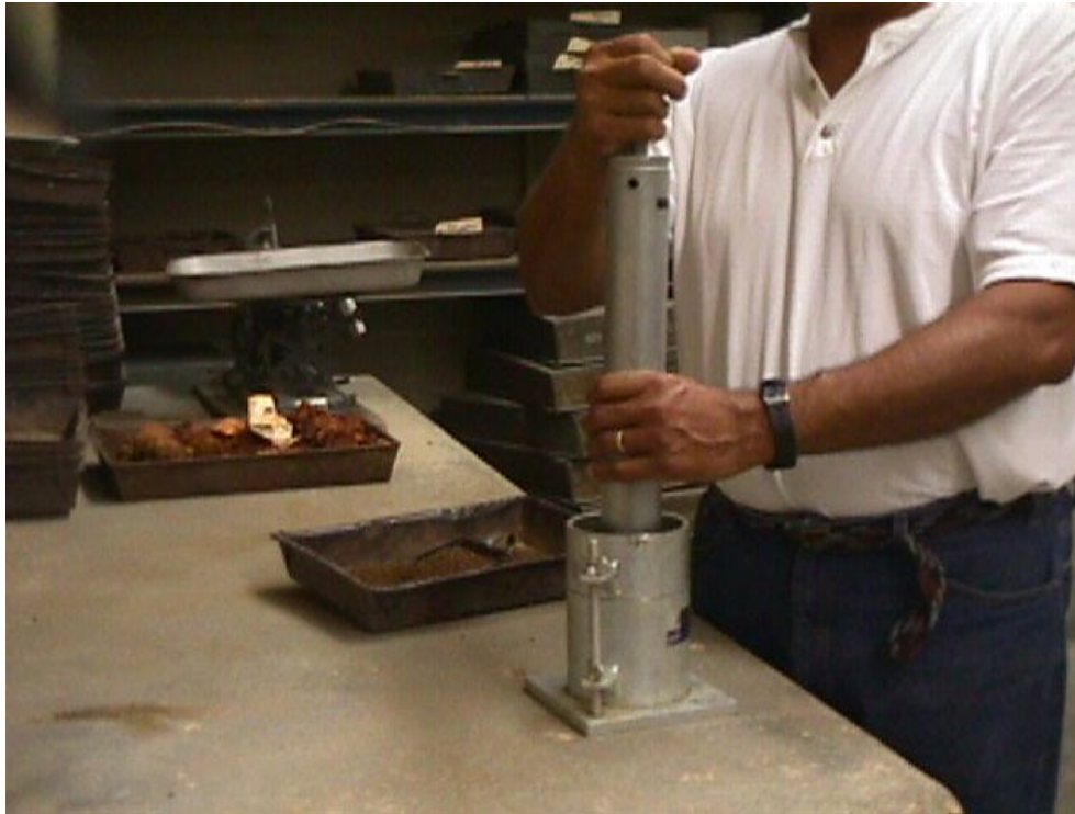
Figure 4: During compaction, technician should keep rammer perpendicular to the sample.
