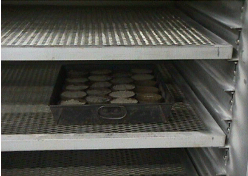
Figure 1: Samples being dried in oven at 110^{\circ} \pm 5^{\circ}\text{C} ( 230^{\circ} \pm 9^{\circ}\text{F} )
