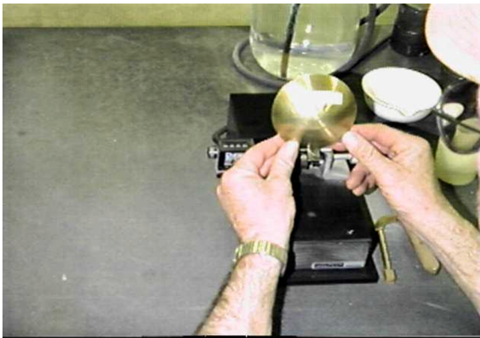
Figure 3: Place a piece of tape which bisects wear spot on bottom of liquid limit cup. This will provide the height gauge with a measuring point.
