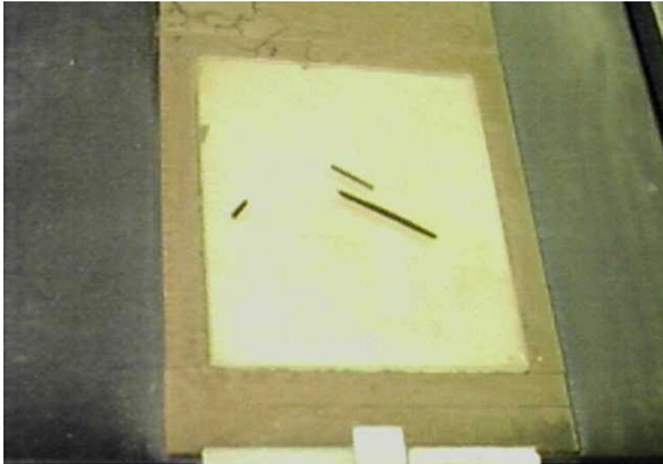
Figure 3: Roll into 3.2 mm diameter thread.
