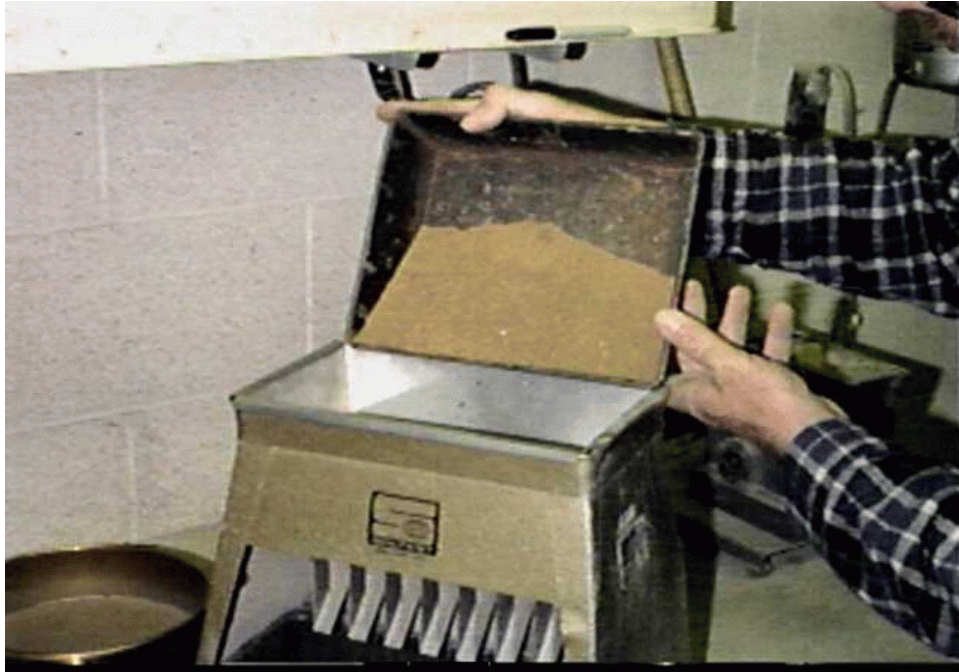
Figure 2: Equal amounts of sample should flow through each chute
