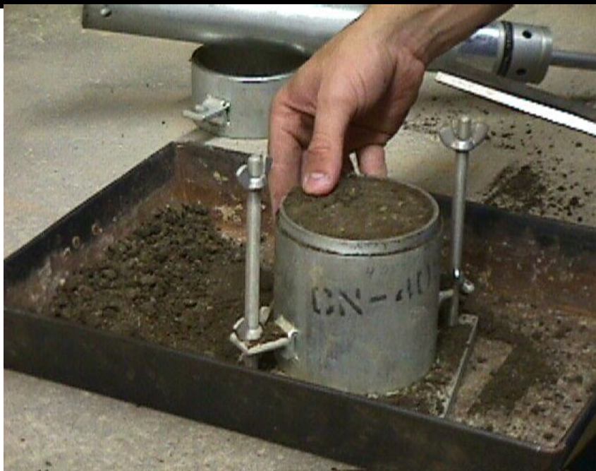
Figure 6: Add soil to any noticeable gaps in soil surface after it has been planed.
