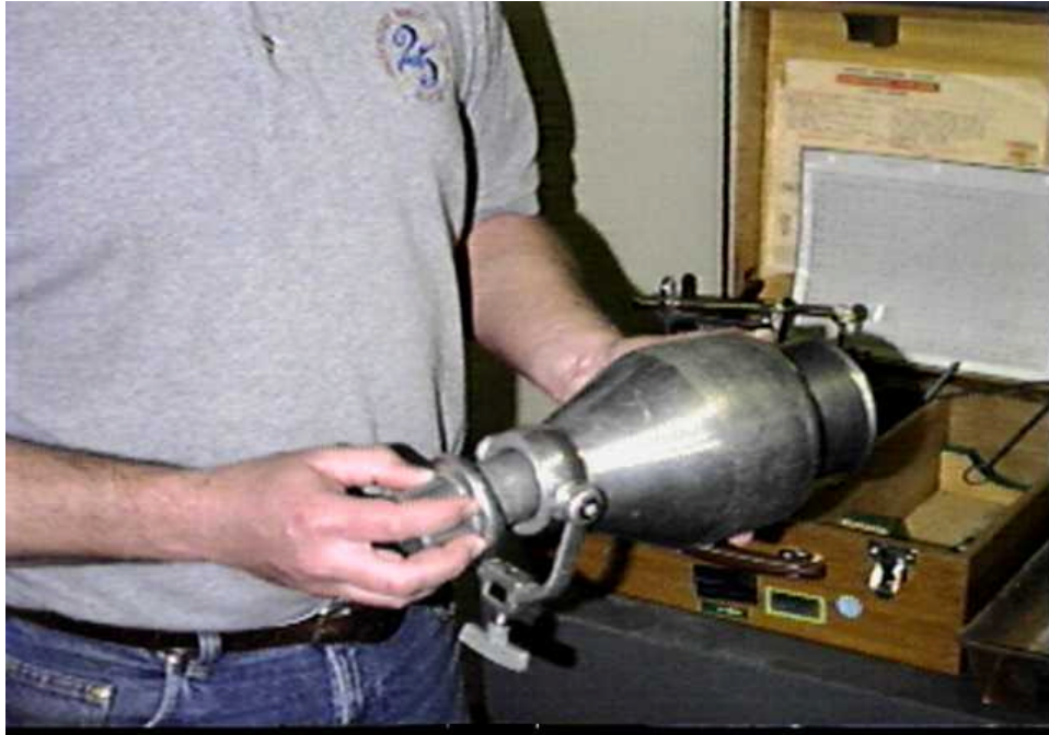
Figure 4. Ensure that seal is made between cap and chamber.
