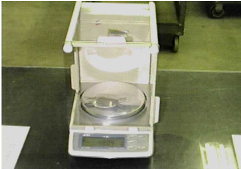
Figure 9: Weigh samples on balance with sensitivity to nearest 0.01g.
