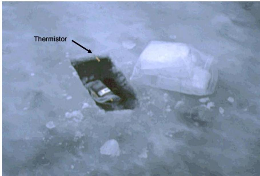
**Figure 9. Ice samples in freezer bag, and thermistor for measurement of in-situ ice temperature.**
