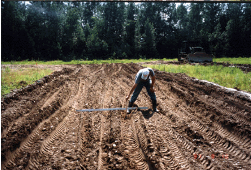
Figure 25. Test section after 30 passes with a 5-ton dump truck.
