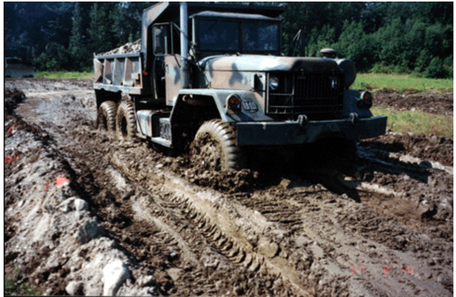
Figure 18. Trafficking the absorbent test section.
