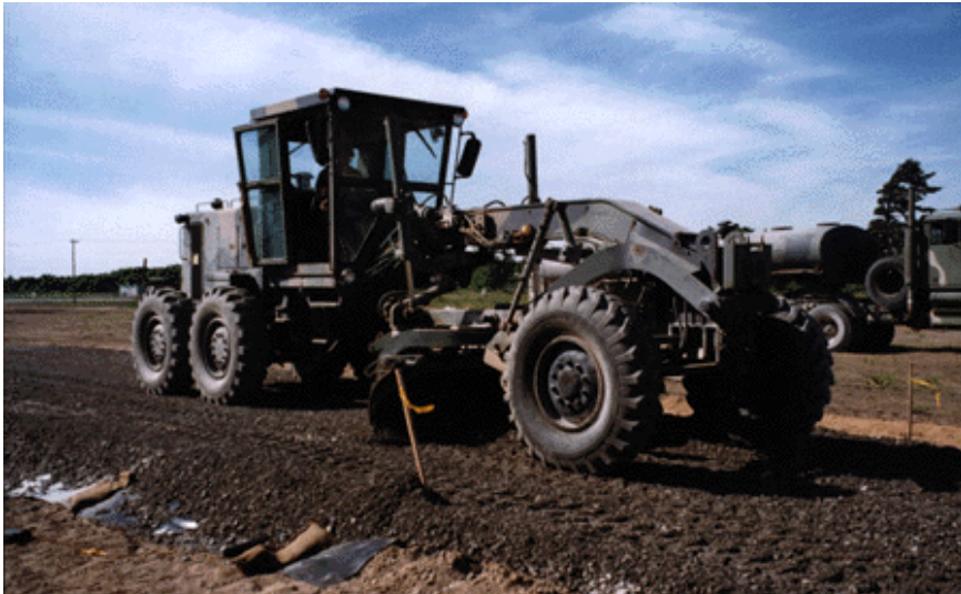
Figure 14. Trafficking the puncture test.
