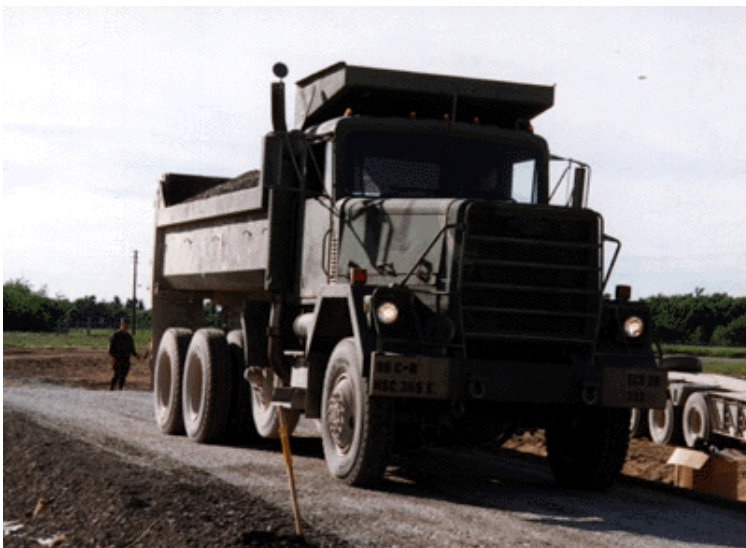
Figure 14. Trafficking the puncture test.
