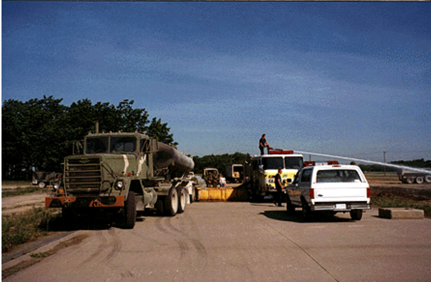
Figure 15. Equipment used to wash gravel off the test section.
