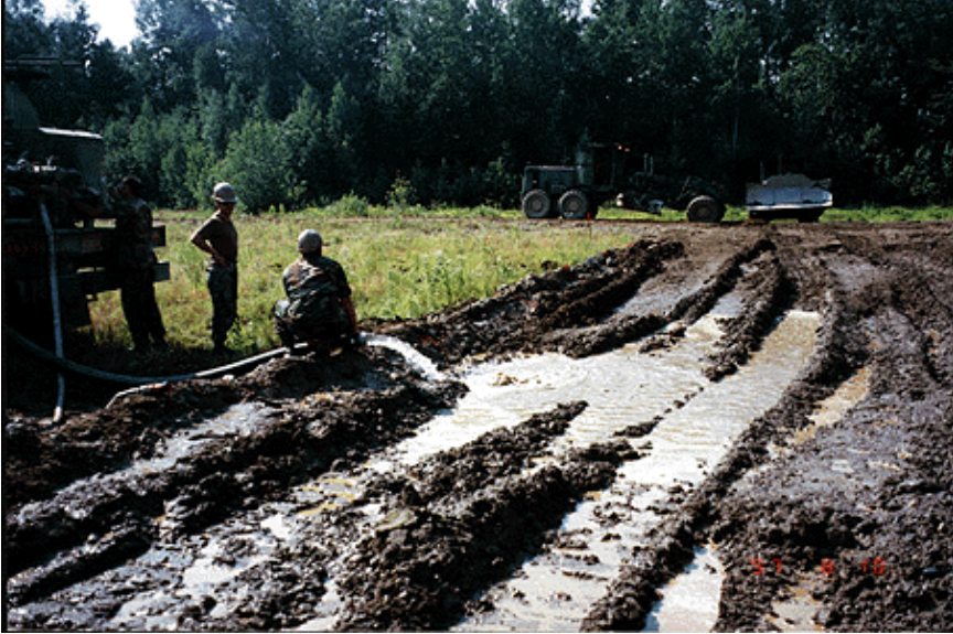
Figure 17. Adding water to the absorbent test section at Ethan Allen Firing Range, Vermont.
