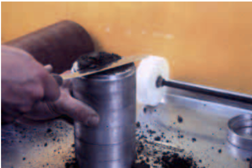
Figure A5. Removal of top layer prior to density–moisture determination.
