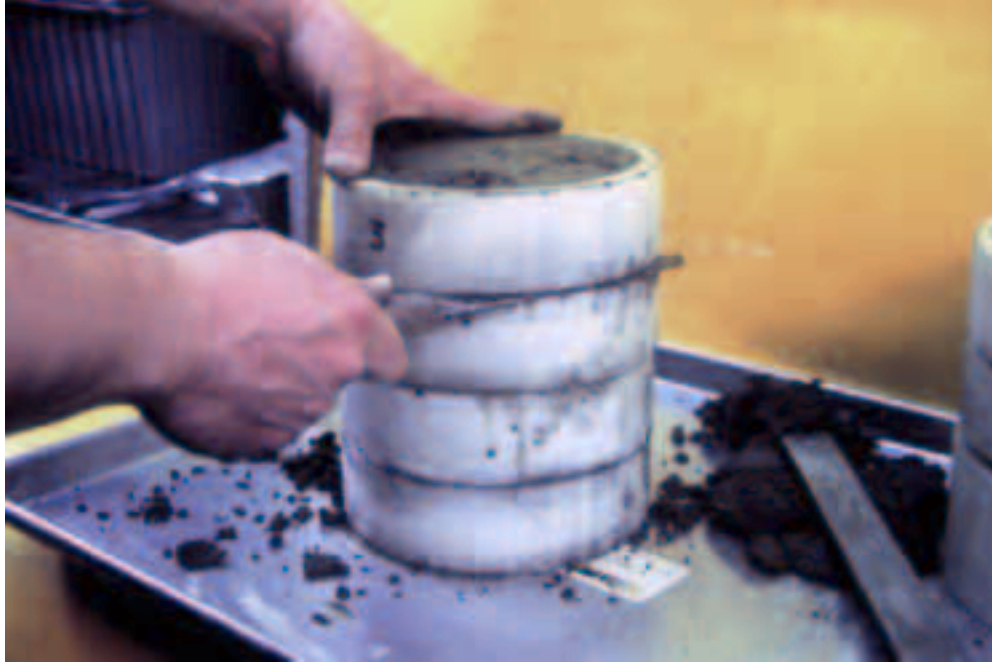
Figure A6. Removal of individual rings for density–moisture determination.
