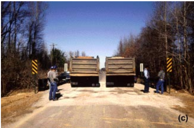
Figure 12—Transverse load test positions used for both load tests: (a) load position 1, 0.6 m upstream of longitudinal center line; (b) load position 2, 0.6 m downstream of longitudinal center line; (c) load position 3, both trucks in same locations as load positions 1 and 2; (d) load position 4, 1.5 m upstream of longitudinal center line; (e) load position 5, 1.5 m downstream of longitudinal centerline; (f) load position 6, both trucks in same locations as load positions 4 and 5.
