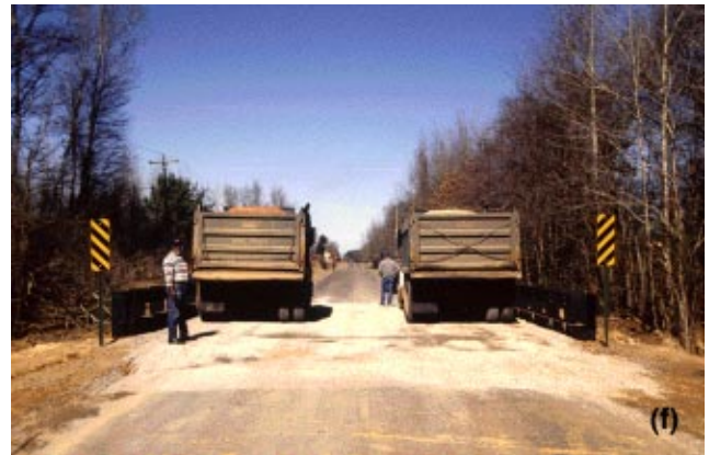
Figure 12—Transverse load test positions used for both load tests: (a) load position 1, 0.6 m upstream of longitudinal center line; (b) load position 2, 0.6 m downstream of longitudinal center line; (c) load position 3, both trucks in same locations as load positions 1 and 2; (d) load position 4, 1.5 m upstream of longitudinal center line; (e) load position 5, 1.5 m downstream of longitudinal centerline; (f) load position 6, both trucks in same locations as load positions 4 and 5.
