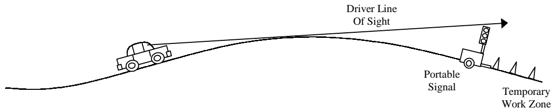
Figure 6. Driver Line of Sight Impeded by Vertical Geometry
