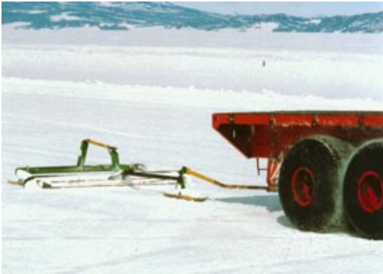
Figure 69. Small snow plane with minor height adjustability.
