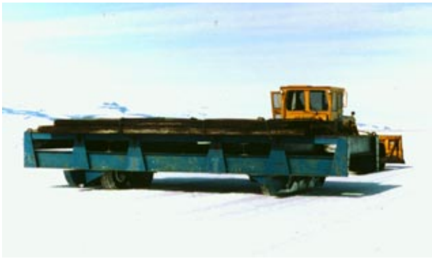
Figure 49. Cart for proof rolling the Pegasus runway shown configured for C-130 landing gear; ballast is steel plate.
