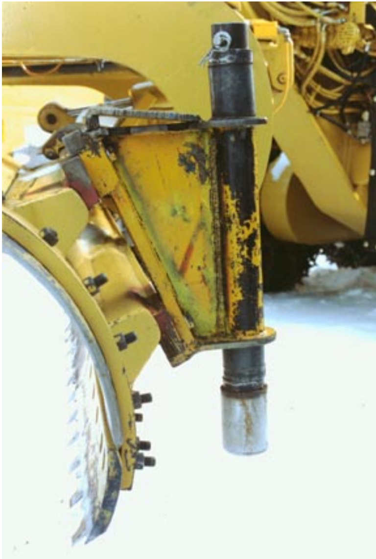
Figure 80. Adjustable skids used to assist in “floating” grader blade.
