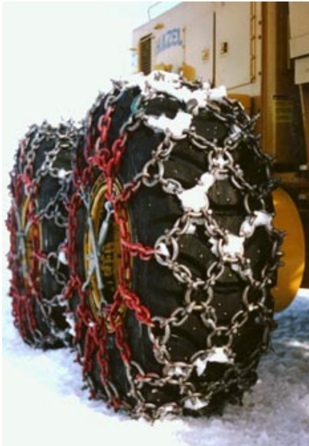
Figure 37. Aggressive tire chains as used in logging industry installed on motor grader to reduce slip during ice grading.
