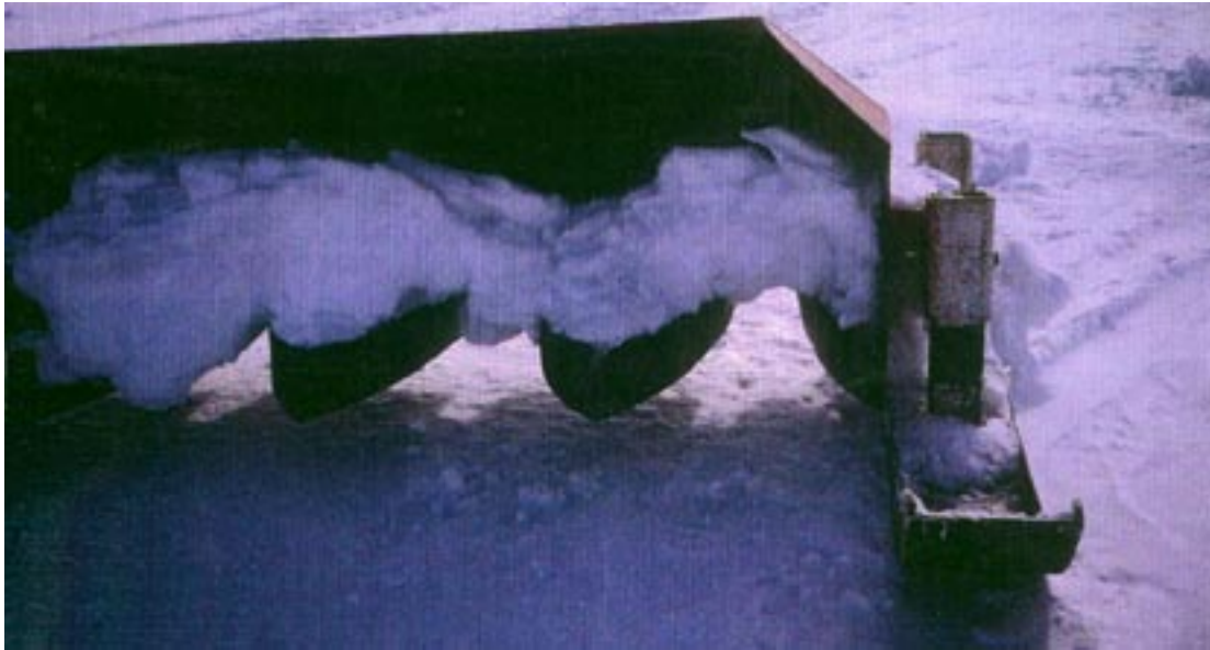
Figure 68. Windrow drag used to encourage snow accumulation.
