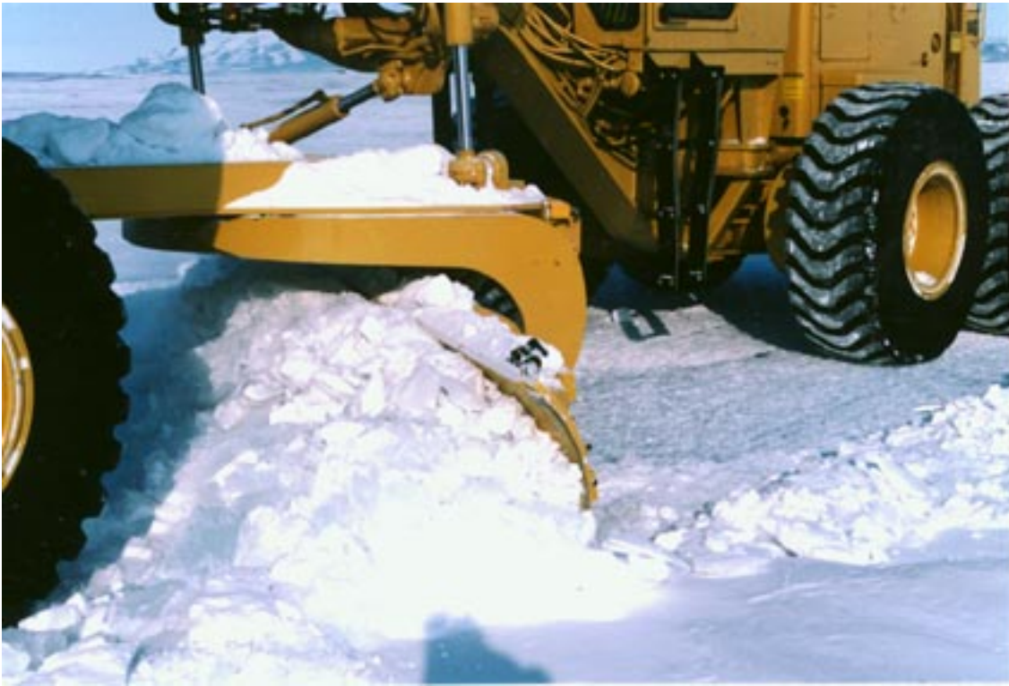
Figure 34. Aggressive grader blade removing up to 20 cm (8 in.) of glacial ice in one pass.
