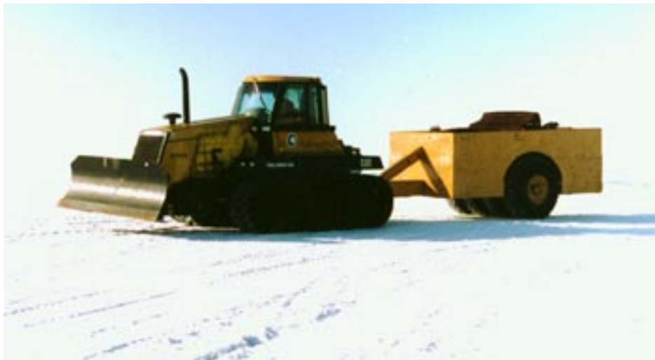
Figure 72. Heavy (45-tonne or 50-ton capacity) pneumatic-tire roller.
