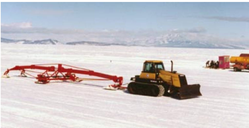
Figure 71. Long-base (12-m, or 40-ft) snow plane with height adjustability.
