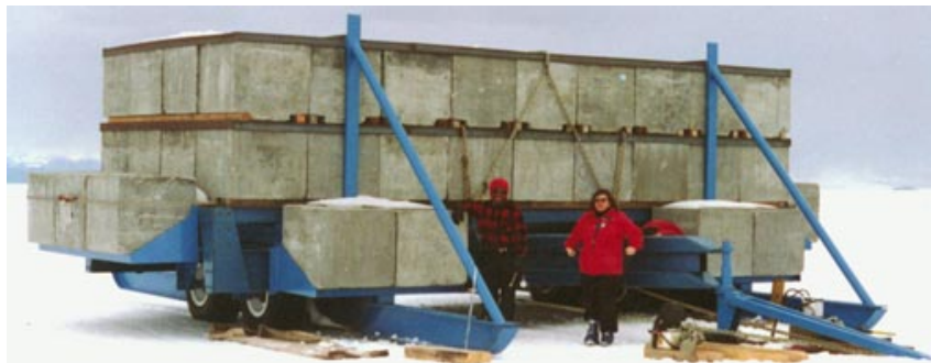
b. Ballasted with concrete blocks.
