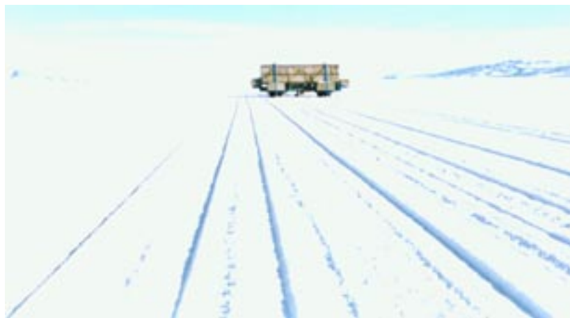
Figure 52. Closely spaced proof cart tire tracks during full-scale load certification of runway.
