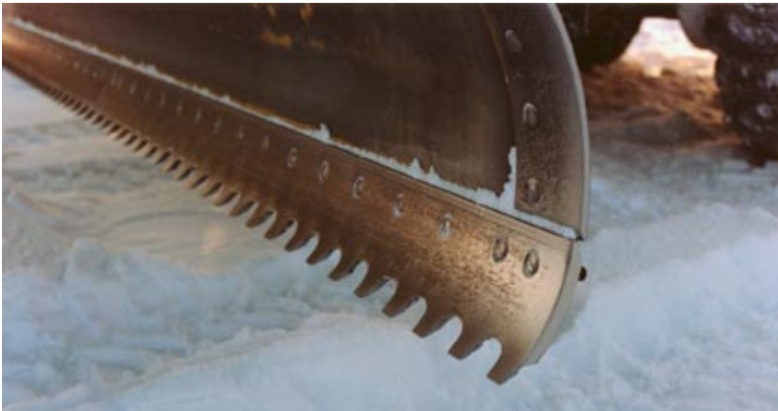
Figure 33. Custom-built aggressive grader blade used for initial rough grading of runway.
