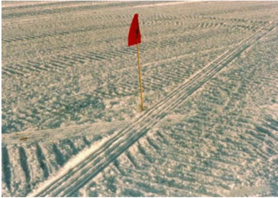
Figure 62. Tracks of proof cart on area patched 48 hours earlier.
