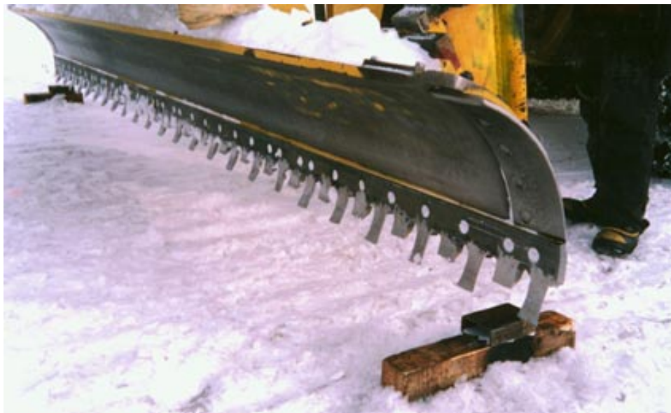
Figure 45. Custom built chisel-tooth grader blade used during finish grading of runway.
