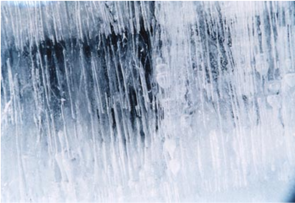
Figure 4. Example of melt/refreeze ice with cylindrical bubbles.
