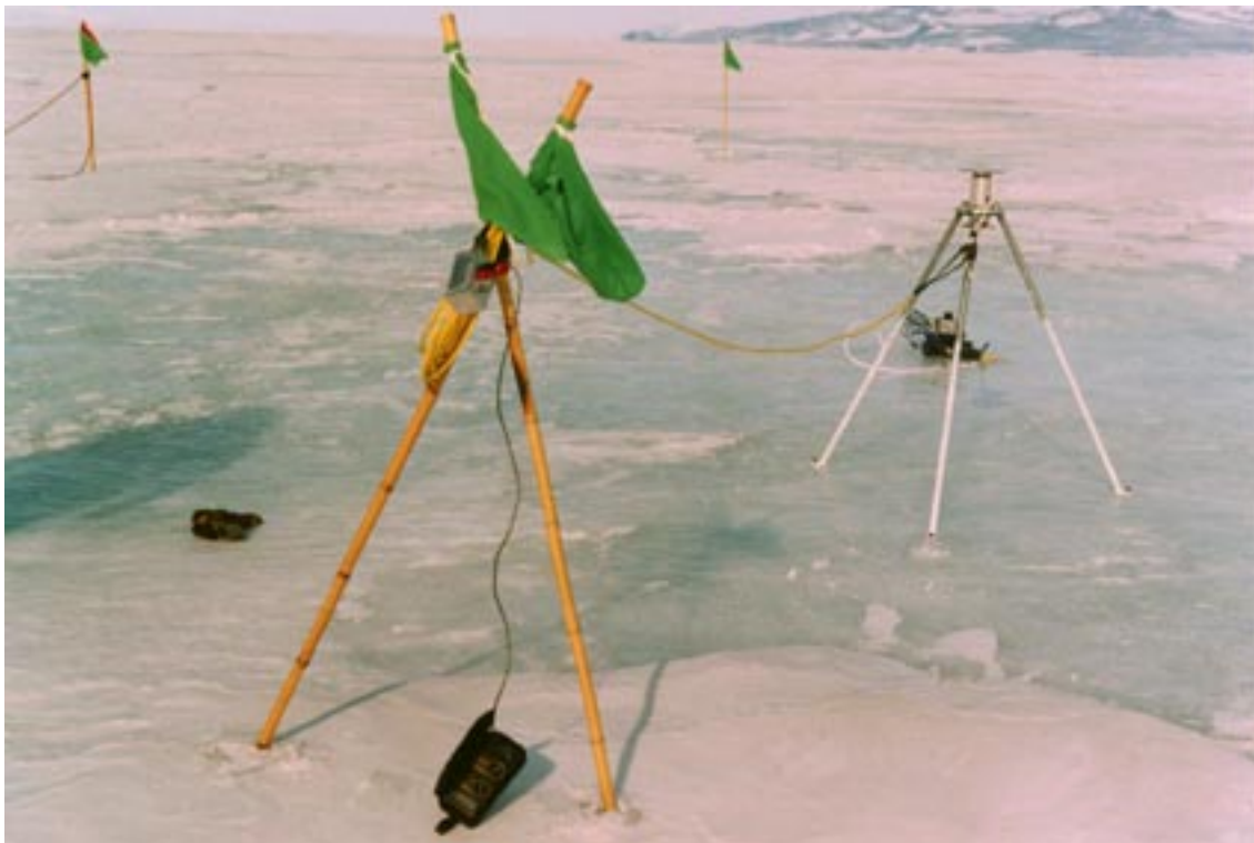
Figure 24. Radiometer pair used to measure albedo of snow and ice surfaces.
