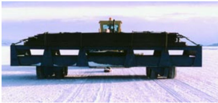
a. Ballasted with steel plate.
