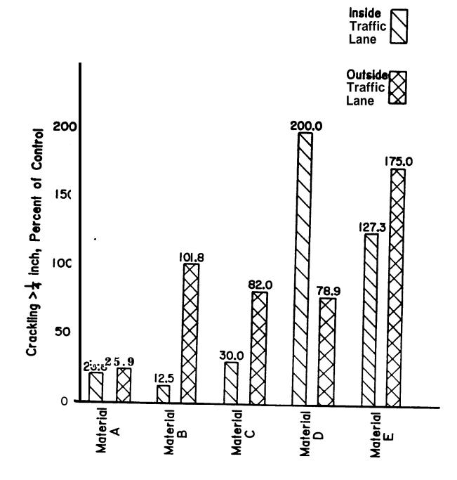
Figure .5.\_ Relationship Between Material Type and Cracking Wider Than 1/4 Inch
