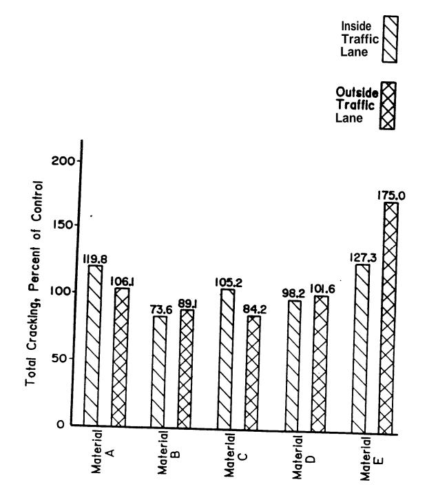
Figure 4. Relationship Between Material Type and Total Cracking
