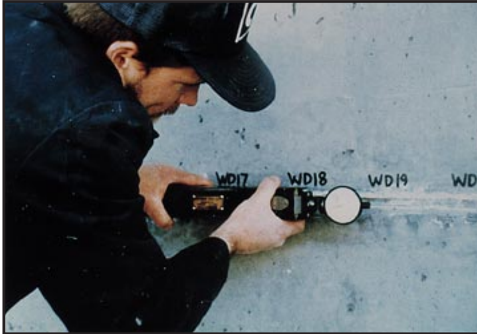
Figure 7. Surface strains. A Whittemore mechanical strain gage is being used to measure transfer length in a prestressed concrete girder.
