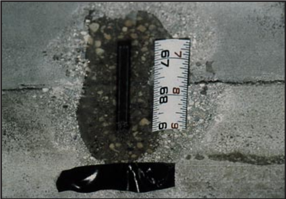
Figure 6. Electrical resistance strain gage on concrete surface. Special preparation on the surface was needed prior to application of the gage.
