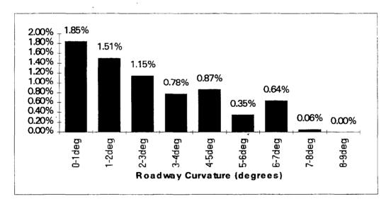
Figure 3-5 Percentage of Rear-End Collisions vs. Roadway Curvature, Weighted (85 NASS)
