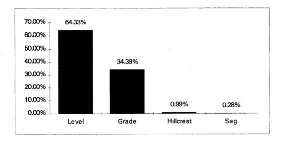
Figure 3-1 Percentage of Rear-End Collisions vs. Roadway Profile, Weighted (85 NASS)
