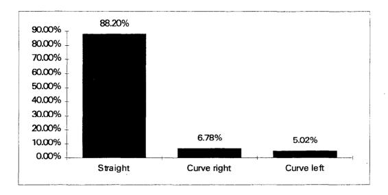
Figure 3-4 Percentage of Rear-End Collisions vs. Roadway Alignment, Weighted (85 NASS)
