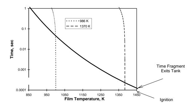
FIGURE 10. FILM TEMPERATURE–TIME HISTORY AND TEMPERATURE–TIME REQUIRED FOR IGNITION IN ULLAGE AT AN ALTITUDE OF 10,000 m ( $V_0 = 237$  m/s, 59 g INCONEL FRAGMENT)
