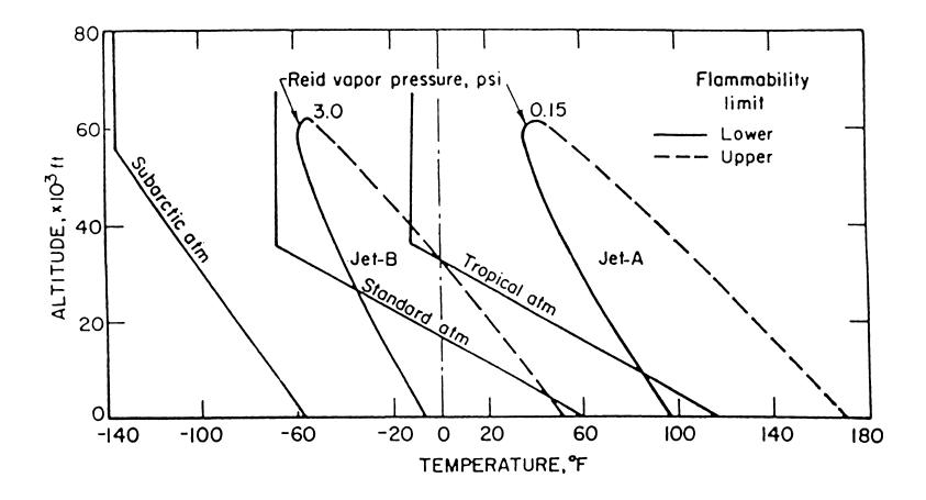
FIGURE 3. PRESSURE ALTITUDE—TEMPERATURE LIMITS OF FLAMMABILITY FOR JET-A AND JET-B TYPE FUELS IN AIR UNDER EQUILIBRIUM (OR STATIC) CONDITIONS (KUCHTA, 1985)
