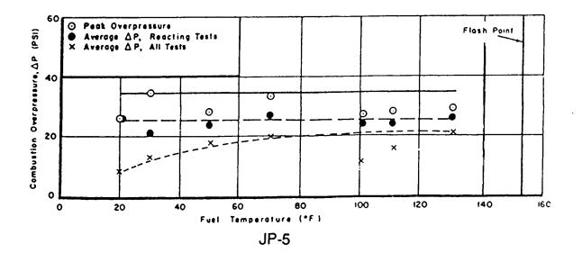
FIGURE 5. COMBUSTION OVERPRESSURE AS A FUNCTION OF FUEL INITIAL TEMPERATURE FOR GUNFIRE TESTS FOR JP-5 AND -8 (90-GALLON TANK, 4-INCH FUEL DEPTH AT ATMOSPHERIC PRESSURE)
