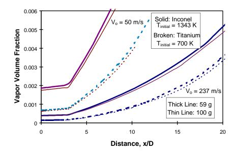
FIGURE 13. MASS FRACTIONS OF VAPOR IN THE WAKE OF A FRAGMENT IN LIQUID FUEL
