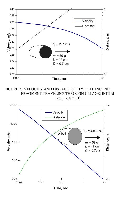
FIGURE 8. VELOCITY AND DISTANCE OF TYPICAL INCONEL FRAGMENT TRAVELING THROUGH LIQUID FUEL; INITIAL  $Re_D = 1.4 \times 10^6$
