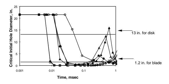
FIGURE 18. CRITICAL INITIAL HOLE DIAMETER ON THE WALL (MAXIMUM ALLOWABLE INITIAL HOLE SIZE AS A FUNCTION OF TIME). THE TWO HORIZONTAL LINES REPRESENT THE INITIAL HOLE SIZE DUE TO THE PERFORATION OF BLADE AND DISK FRAGMENTS.
