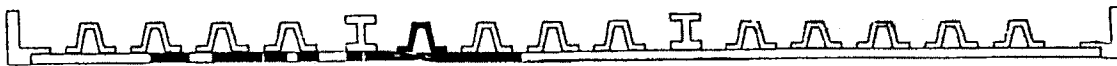
Figure 4. Damage of Skin at the Doubler Edge on Wing Lower Surface: V95T Alloy; \sigma_{\text{fract net}} = 0.45 \sigma_{0.2} ; K_{\text{fract}} = 0.5 K_c^{\text{app}} .
