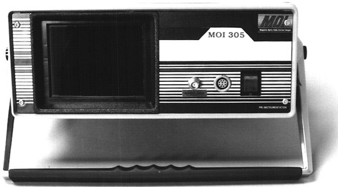
FIGURE 8. THE MOI 305 PROTOTYPE POWER UNIT
