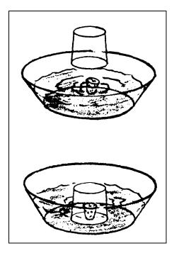
Remove the glass and the cork. Stuff facial tissue into the bottom of the glass. Invert the glass and push to the bottom of the bowl. The tissue doesn't get wet.
