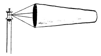
The large end of the sock will catch the wind, so that the small end will point away from the direction from which the wind is blowing, or will droop if there is not enough wind to keep it extended.
