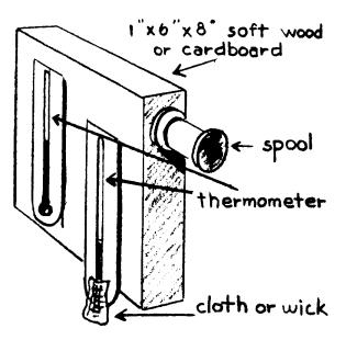
To make a sling psychrometer, remove the metal guard from one thermometer and cover its bulb tightly with the cloth or wick. Nail both the thermometers onto the board. Using the nut and bolt, attach the spool to the upper corner of the board, so that it will rotate freely.
