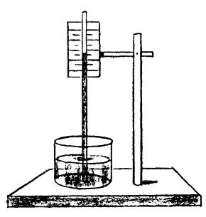
Mark a scale of inches and half inches on the cardboard, and label it from 24 to 36 inches. With the yardstick, measure the actual height of the mercury column and attach the scale to the proper spot on the tube.
