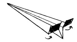
Fold the back edges of the glider*down*. When you throw the glider, the tail should go up and the nose should go down. This same thing happens when the pilot tilts the elevators downward.
