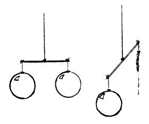
Blow up the balloons to the same size, and tie them at their necks with a piece of string. Tie one balloon to each end of the dowel stock. Attach another piece of string to the center of the dowel stock and suspend it from some convenient place. Balance the dowel stock. Prick one balloon with a pin. As the air rushes out, the pricked balloon shoots up and the heavier, air-filled one drops down.
