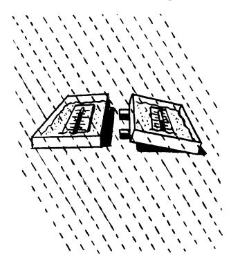
The tilted thermometer records the result of the direct rays of the sun which represent the direct rays of summer. The level thermometer records the angular rays of winter. The tilted thermometer should have a higher reading than the level thermometer. It is possible to obtain a greater contrast of angle, and therefore of temperature readings, when this demonstration is performed in winter.
