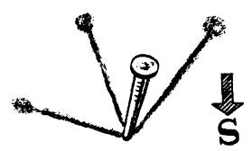
Put nail in the board centered near one edge. Mark an S at edge of board in front of the nail. Place the board in a spot which will have sun all day, being sure that the edge of the board with the S and the nail are facing south. Mark along the line of shadow every hour on the hour.
