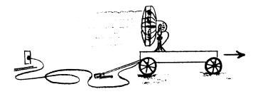
Put a propeller on anything that can move-a wagon or a roller skate. Use a small electric fan with a very long extension cord for a propeller. Set it firmly on the roller skate or wagon. The fan drives the wagon or skate backwards. This is because the blades are set to throw the air in front of the fan.
