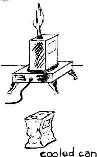
When it was heated water turned into steam, driving out most of the air. Now as the can cools, the steam turns back into water, leaving neither air nor steam inside the can. A partial vacuum has been created. Consequently, the pressure of air outside the can, being greater than that inside the can, crushes the can.
