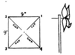
Experiment to see whether there is any angle toward the wind at which you might hold your pinwheel without it spinning. When does it slow down? Is it when the plane of the blades is parallel to the wind? Each blade is an airfoil. Can you explain why? (See No. 42.)
