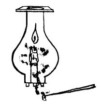
Light the candle and place the chimney over it, resting the chimney on sticks so thatair can circulate under the edge. Put the cover glass over the top of the chimney. Light the splinter and hold it near the base of the candle so that smoke will circulate inside the chimney.
