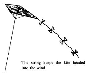
The tail keeps the kite upright. Gravity tends to pull the kite down.
