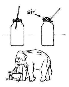
straw with clay. Put the cap on tightly so that no air can get into the bottle. Now try to suck the water out of the bottle. No matter how hard you suck, the water will not flow through the straw. Release the cap on the bottle just enough to let in some air, and try to suck the water through the straw. Now, as you suck through the straw, the air pressure is lowered inside the straw. Air pressing on the surface of the water in the bottle pushes it up through the straw as you suck through it.
