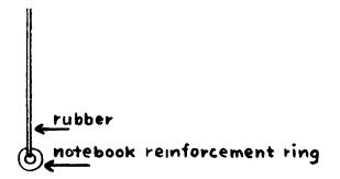
Fasten this end to the glider as shown in the diagram below; then anchor with a pin. Even kindergarten children can use this method of suspending a glider in a wind tunnel. (See No. 55.)
