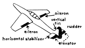
a. *Up and down*. Fold the back edges of the paper glider *up*, as in the diagram. When you throw the glider, the tail should go down and the nose should point up. It may take some practice to get the controls set so the glider does what you want it to do.
