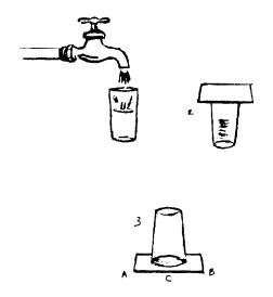
At A and B the upward and downward pressures balance, but at C the upward pressure of air is greater than the downward pressure of water and holds the cardboard in place.
