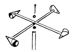
The anemometer may be calibrated with a fair degree of accuracy as follows: Hold it out the window of an automobile moving at a constant rate of speed. Note the speedometer reading and the distance traveled and the revolutions per minute (rpm) of the anemometer. Drive the car back along the same road and note the same readings, being sure the speed of the car and the distance traveled are the same as before. Average the 2 rpm counts to allow for the effect of any wind.
