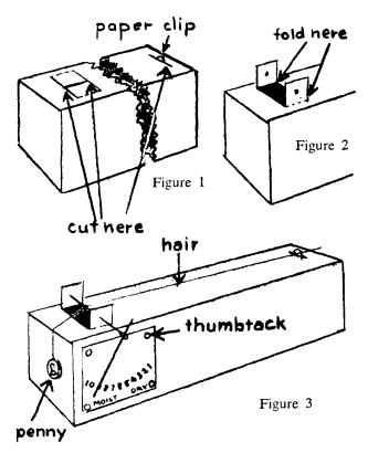
Tie the hair to the paper clip, wind it around the needle, tape the penny to the other end of the hair, and let the penny hang over the end of the box, which should be lying on its side.
