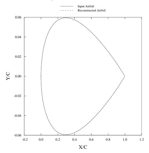
Input/Reconstructed NACA 0012 Airfoils
