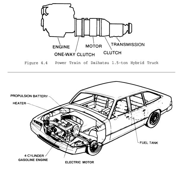
Figure 4.5 Schematic of DOE's Hybrid Test Vehicle HTV-1
