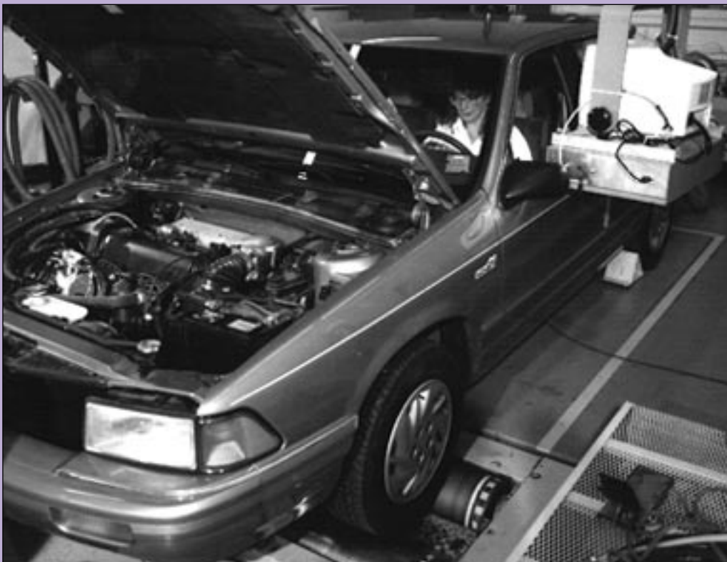
With a chassis dynamometer, the drive wheels of a test vehicle are supported by rollers that simulate driving conditions. Fuel economy and emissions are measured while driving on the dynamometer.
