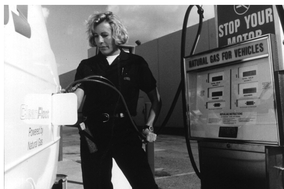
Figure 12. The natural gas fueling station had two compressors, cascade storage, and a dispenser.
