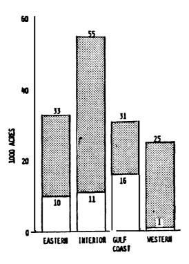
Figure 1-2: Surface area requirements for coal strip-mining over a 30-year lifetime for a 50,000 bbl/day plant.
