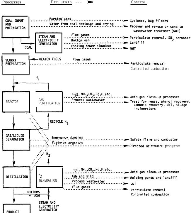
Simplified Direct Liquefaction Process-waste Stream Figure 2-1: Sources and Control
