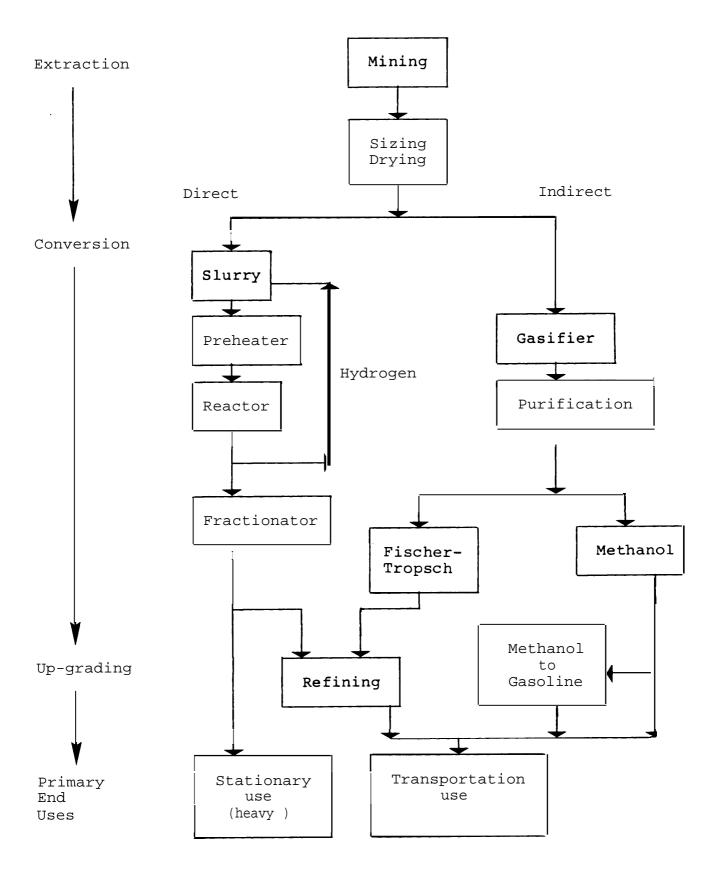
Figure 1-1: Coal Liquefaction Process Steps
