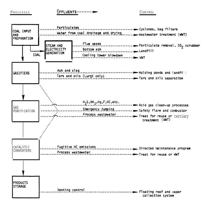
Figure 2-2: Simplified Indirect Liquefaction Process-waste Stream Sources and Control
