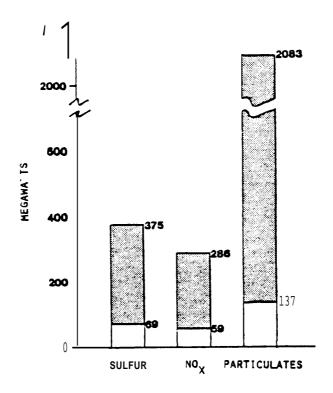
Figure 1-4: Size ranges of coal-fired power plants with emissions equal to 50,000 bbl/day synfuel plants.
