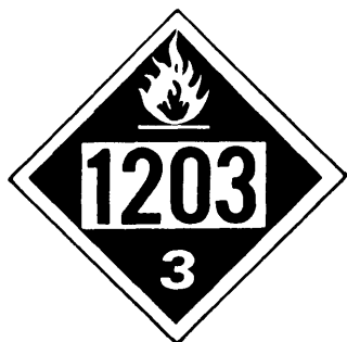
Photo credit: Office of Technology Assessment based on 49 CFR 172.332 1203 is the UN/NA identification number for gasoline.
