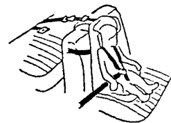
Fig. 2 Tether attached to rear safety belt
