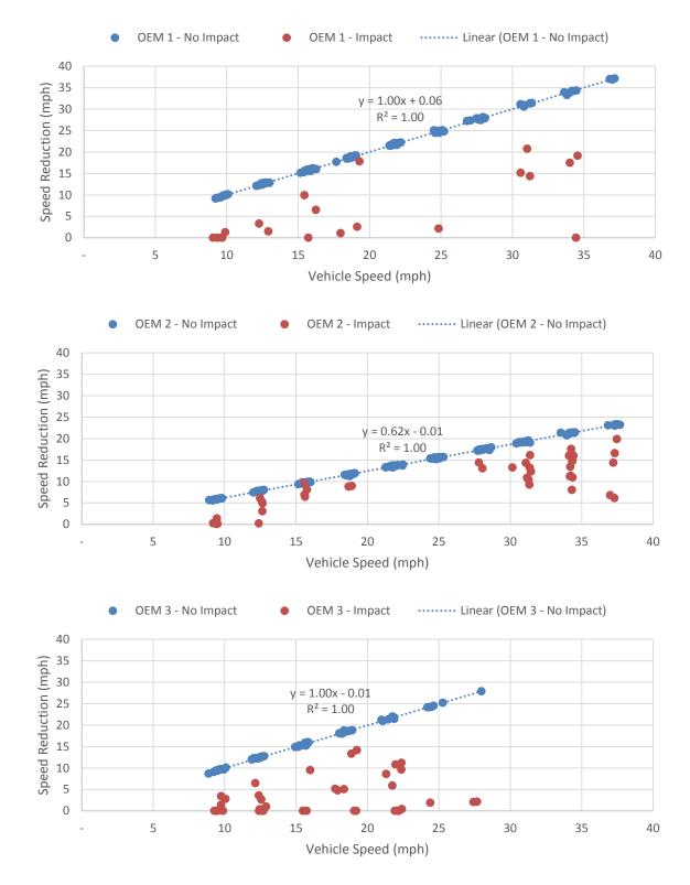
Figure 9: Test Results With Only AEB Active, Comparing Speed Reduction for an Adult Walking in S1 During the Day With No Obstruction for All Three OEMs
