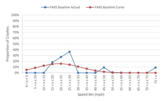
Figure 30: Plots of Normal Distribution Function Compared to Actual FARS Data for a Child Walking in S1 During the Day With an Obstruction
