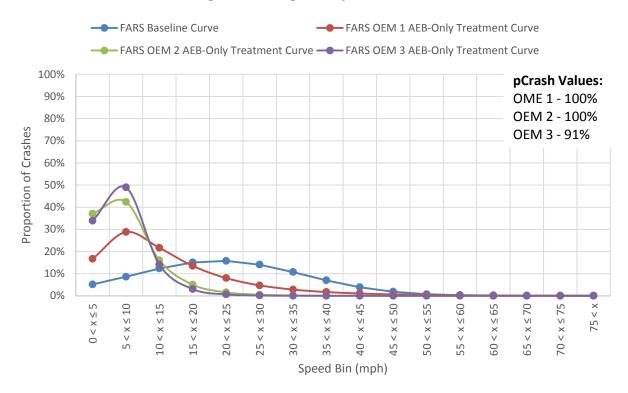
Figure 41: Plots of Functions Comparing FARS Baseline to FARS Treatment for AEB Only Results Data for a Child Walking in S1 During the Day With an Obstruction for All OEMs
