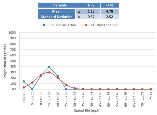
Figure 29: Plots of Normal Distribution Function Compared to Actual GES Data for a Child Walking in S1 During the Day With an Obstruction
