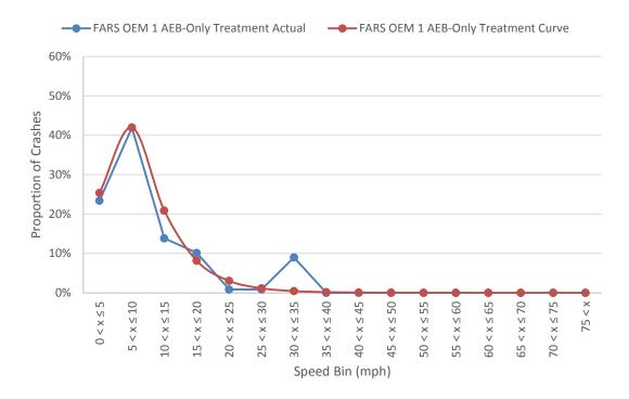
Figure 16: Plots of Log Normal Distribution Function Compared to Actual FARS Data for an Adult Walking in S1 During the Day With No Obstruction for OEM 1, Under the AEB Only Treatment
