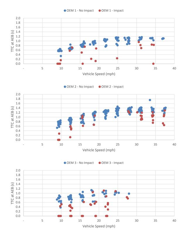
Figure 8: Test Results With Only AEB Active, Comparing AEB Activation Time for an Adult Walking in S1 During the Day With No Obstruction for All OEMs
