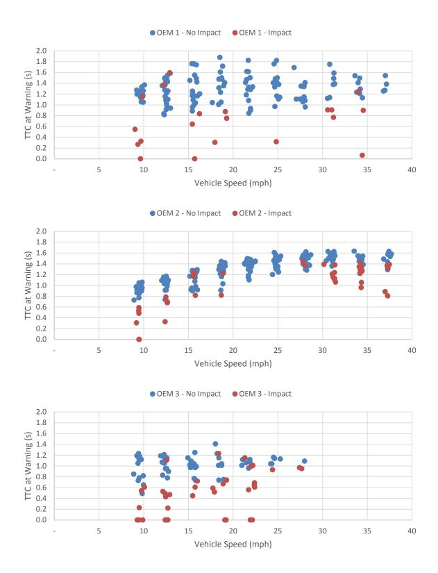
Figure 7: Test Results With Only AEB Active, Comparing TTC at Warning for an Adult Walking in S1 During the Day With No Obstruction for All OEMs
