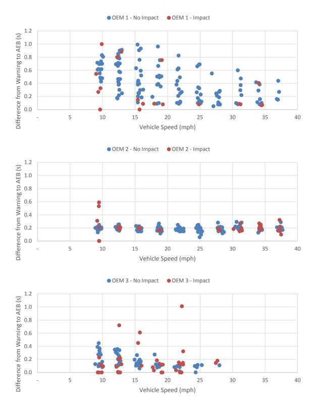
Figure 12: Test Results With Only AEB Active, Comparing Difference From Warning Time to AEB Activation for an Adult Walking in S1 During the Day With No Obstruction for All OEMs
