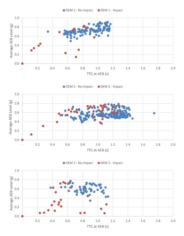
Figure 11: Test Results With Only AEB Active, Comparing AEB Activation Time From OEM 2 for an Adult Walking in S1 During the Day With No Obstruction
