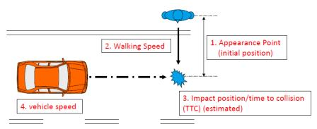
Figure 23: Parameters Needed for an S1 Crash Reconstruction [10]
