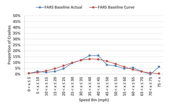
Figure 20: Plots of Normal Distribution Function Compared to Actual FARS Data for an Adult Stationary in S4 During the Day With No Obstruction, Under the AEB Only Treatment
