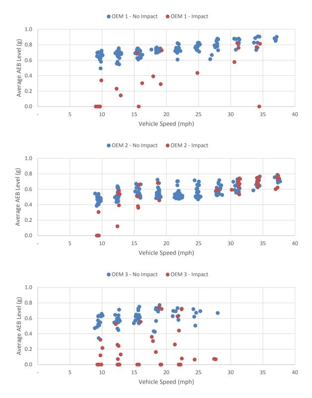
Figure 10: Test Results With Only AEB Active, Comparing Average AEB Level for an Adult Walking in S1 During the Day With No Obstruction for All Three OEMs
