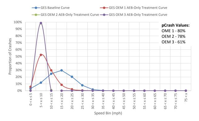
Figure 40: Plots of Functions Comparing GES Baseline to GES Treatment for AEB Only Results Data for a Child Walking in S1 During the Day With an Obstruction for All OEMs
