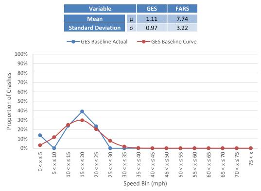
Figure 27: Plots of Normal Distribution Function Compared to Actual GES Data for a Child Walking in S1 During the Day With No Obstruction
