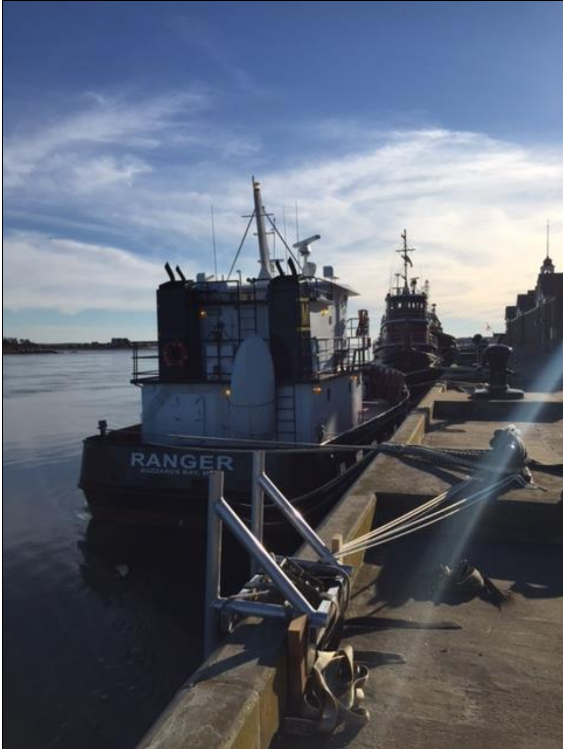
Figure A-10: Photograph of the H-ADCP mounting structure relative to the M/V Ranger following installation of both systems. The Aquadopp Profiler was mounted outboard of the vessel about midships (blocked from view, see Aquadopp report dated March 16). The H-ADCP was mounted at a distance of about 20m-25m laterally along the pier from the Aquadopp.
