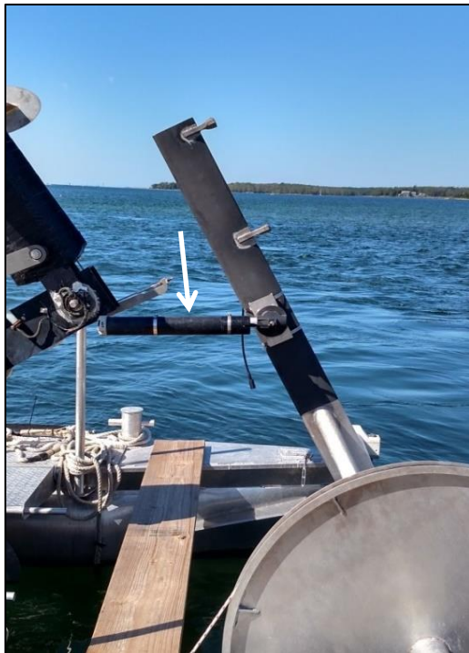
Figure 3: The Aquadopp Profiler is shown (white arrow) strapped to the strut mounting bar on the bow of the Joule device. The strut was in the upright position at the time of this photograph – it was then rotated into the water such that the strut was oriented vertically, and the Aquadopp inclined at a 65° angle from the vertical.
