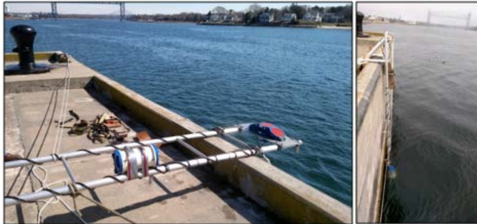
Figure 24. Horizontal water current profile measurement.
