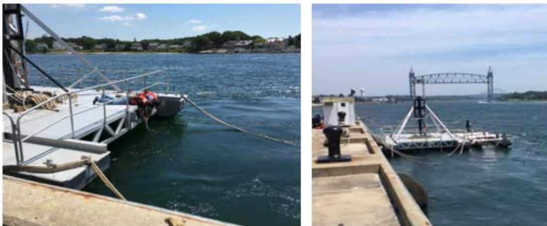
Figure 34. Photograph of the hydrophone mounting location. The hydrophone was mounted on a pole to the back of the MMA barge between the pier and the Leading Edge prototype (the Joule), submerged ~1.5-2 feet below the surface of the water.
