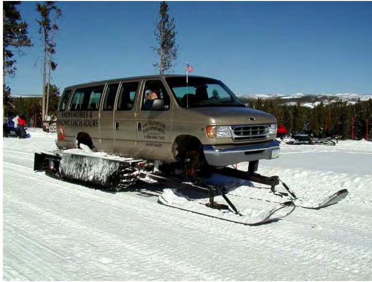
Figure 17: Two-track / full-track / Snow Buster conversion van snowcoach, Reference 9
