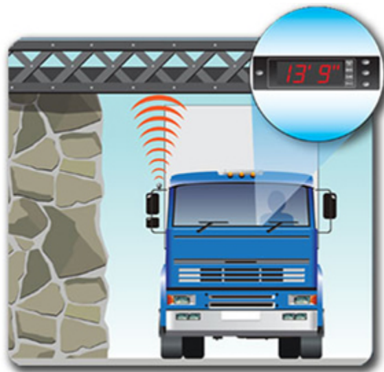
Figure 4. Operation of Giraffe 4 Sonic Bridge Height Measurement
