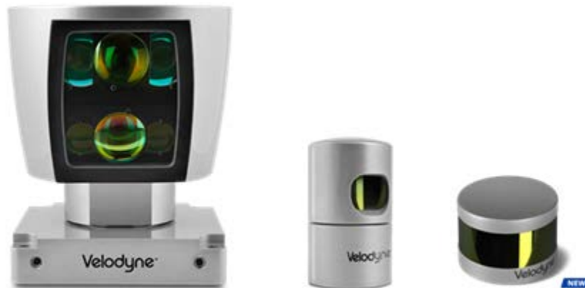
Figure 10. Velodyne LIDARS - HDL-64E (left), HDL-32E (center), VLP-16 (right)
