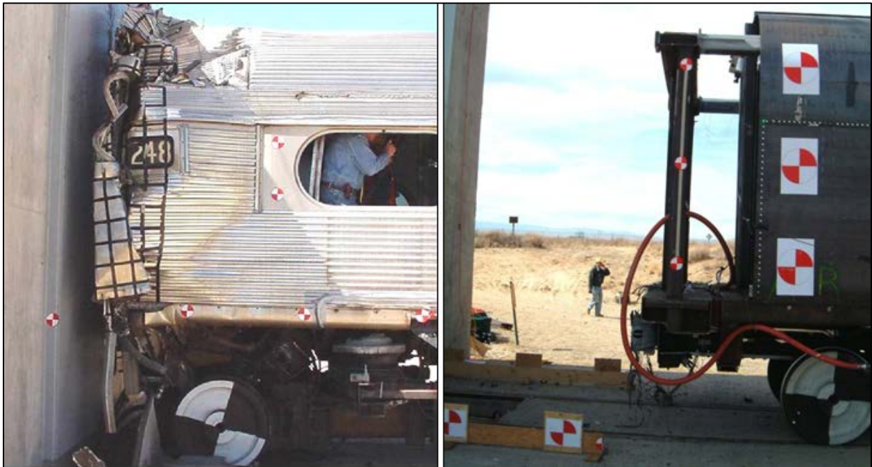
Figure 11. Post-Test Photographs of Conventional (left) and CEM (right) Vehicles
