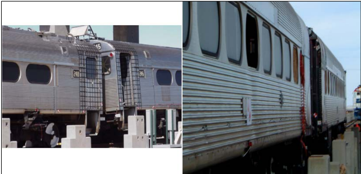
Figure 12. Post-test Photographs of Conventional (top) and CEM (bottom) Coupled Connections
