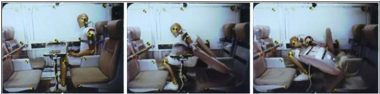
Figure 27. Photo Series for Experiment 1-3, THOR with Table, Leading Car
