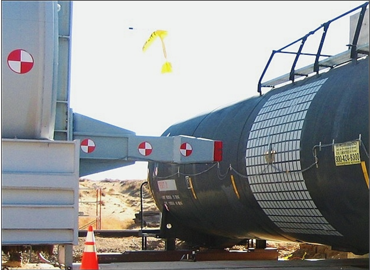
Figure 6. Ram Arm with 12- by 12-inch Indenter Aligned with Center of the Tank Car
