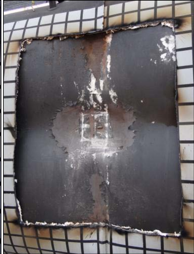
Figure 14. Tank Car Indentation – Removed Jacket and Insulation Section
