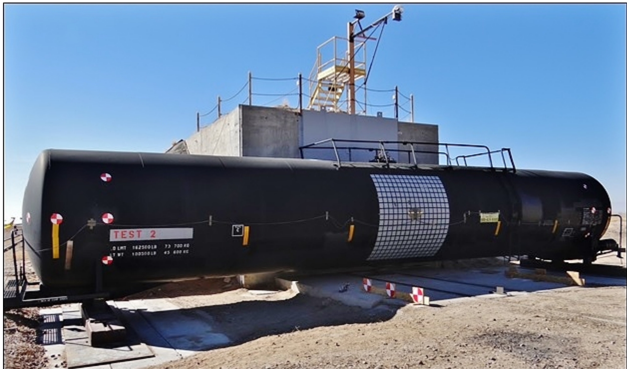
Figure 2. Target Tank Mounted on Support Skids
