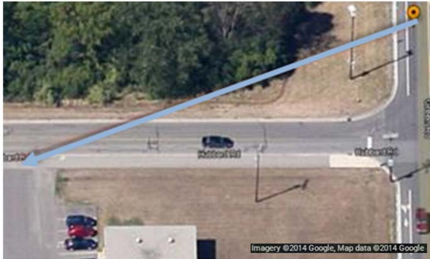
Figure 30 – IMA Scenario Examples: RV or HV Can Comfortably Brake to Avoid Collision (Imagery ©2014 Google, Map data ©2014 Google. Used with permission.)
