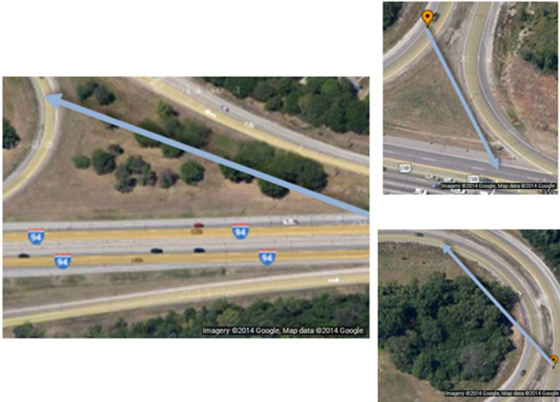
Figure 28 – IMA Scenario Examples: HV on Ramp (Left); RV on Ramp (Top Right); HV and RV Both on (Non-intersecting) Ramps (Lower Right)
