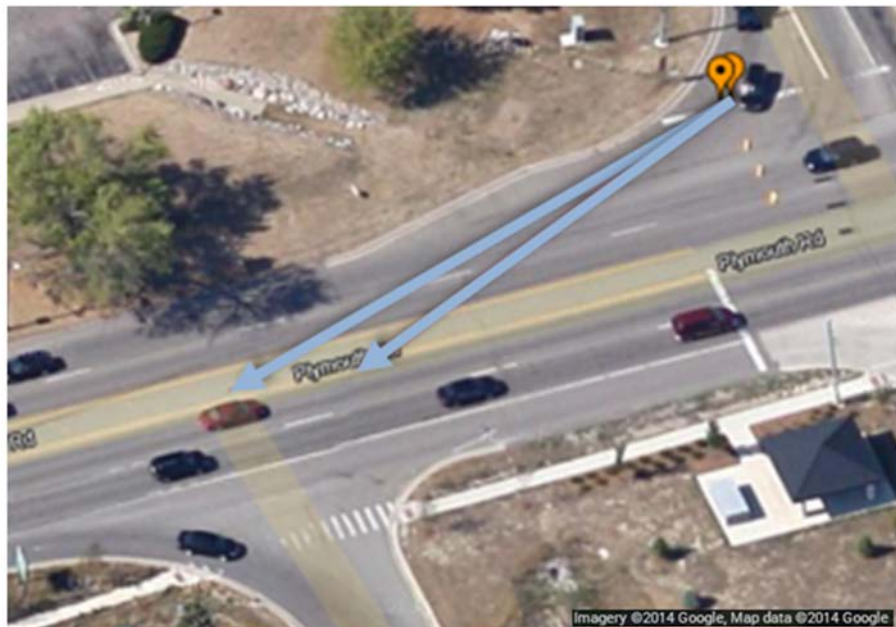
Figure 33 – IMA Scenario Examples: HV Stopped While RV Was Turning Right Onto Far Lane
