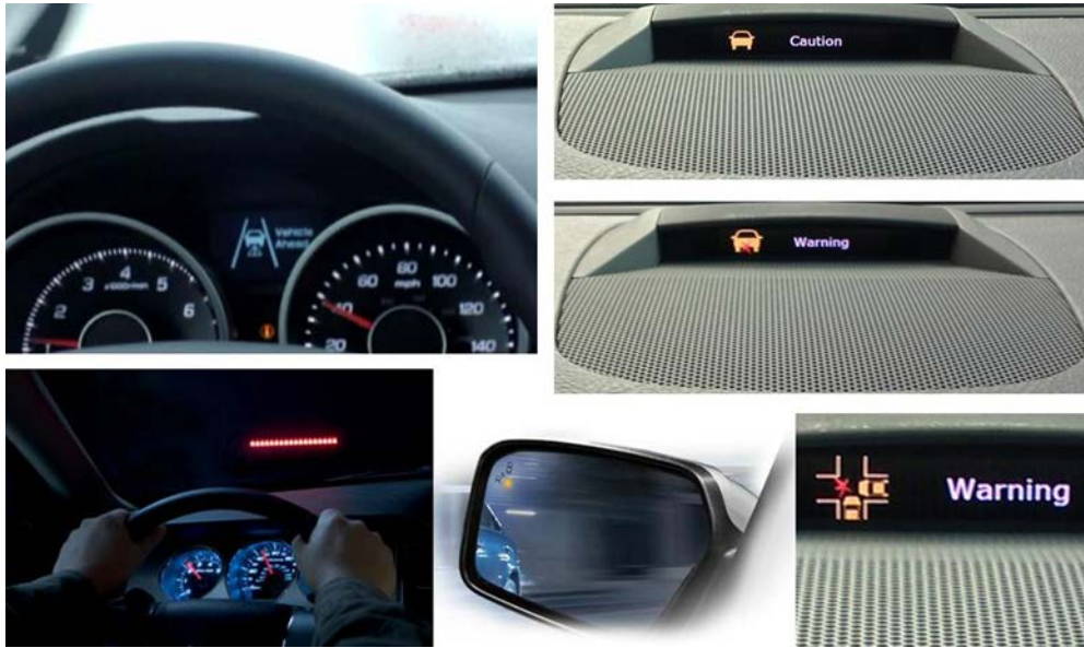
Clockwise from upper left: an FCW alert; an FCW caution; an FCW imminent; an IMA; an LCW; an FCW.
